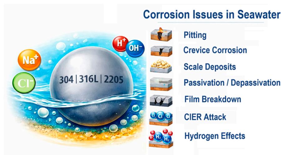
Figure 6. Schematic overview of corrosion mechanisms affecting stainless-steel electrodes during seawater electrolysis.
