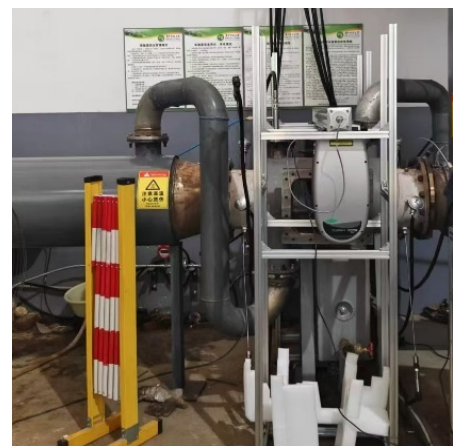
(b) Arrangement of the particle size analyzer on the test bench
