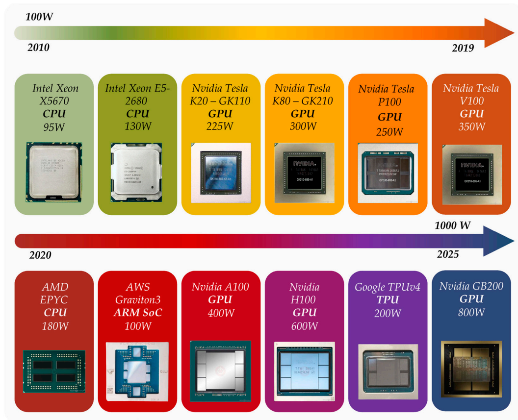
Figure 1. Generations of widely used chips in data center servers. Chip graphics from manufacturer datasheets and www.techpowerup.com ©. The power rating growth trend is visible especially with the advent of AI/ML workloads and GPUs and TPUs becoming the main workhorse of AI servers (Power ratings based on chip maximum TDP).
