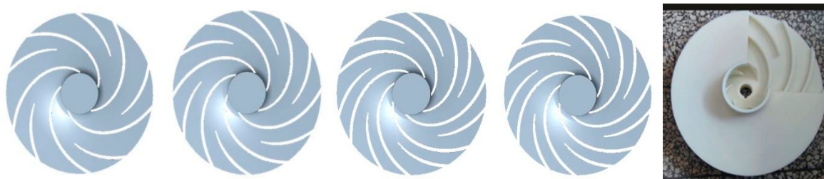
Figure 3. Three-dimensional hydraulic model diagram of impellers with different numbers of split blades.
