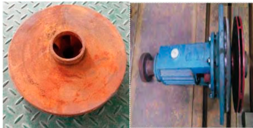
Figure 1. Pump as turbine model.
