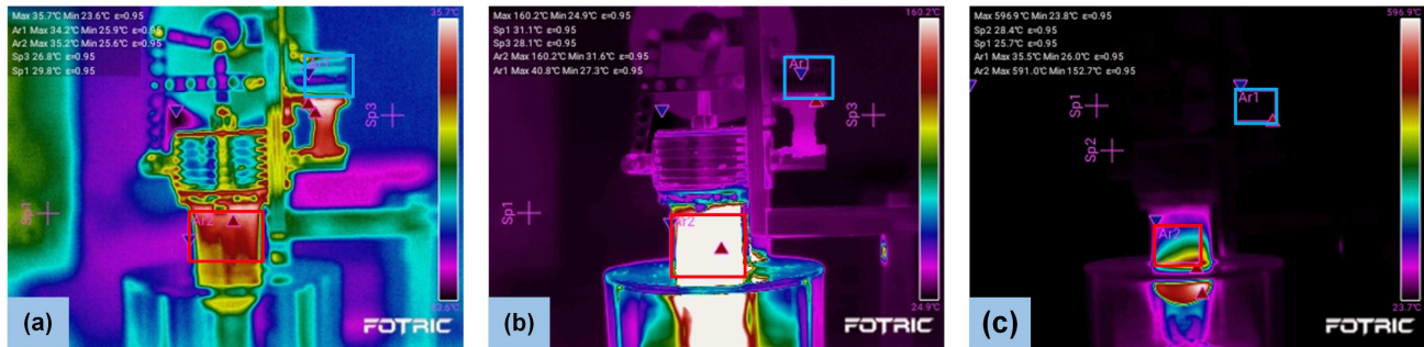
Figure 4. Infrared images of the Stirling engine at different operating stages. (a) Before starting; (b) starting rotation; and (c) output saturation. The red and blue boxes indicate the temperature measurement regions of the hot and cold chambers, respectively. The red \triangle and blue \nabla mark the highest and lowest temperature points within the selected regions.
