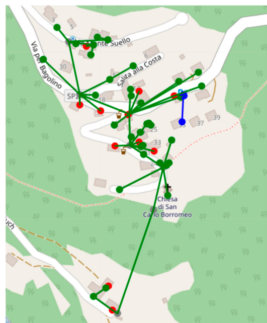
Figure 13. Riccomassimo distribution network on OpenStreetMap. The green circles and lines indicate, respectively, the LV consumers' buses and lines; the red circles are the prosumers' and producers' buses, while the blue circles and lines indicate the transformer.
