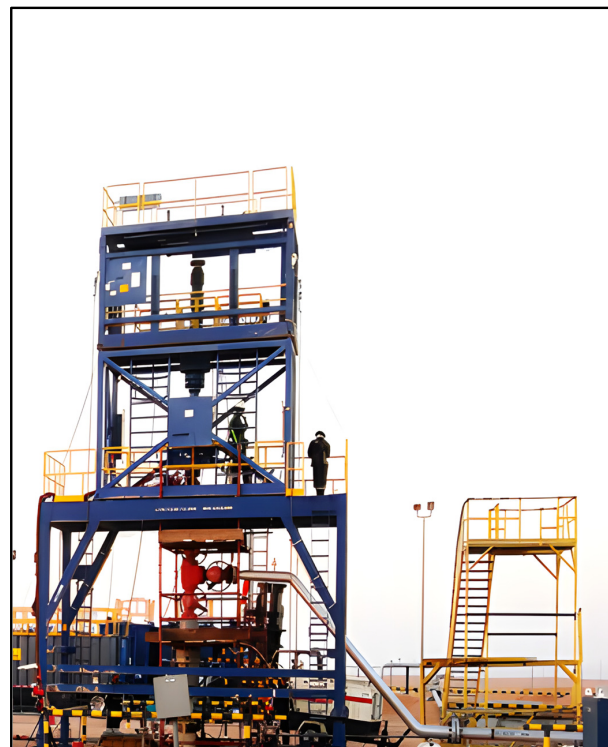
Figure 7. Image of tower system (left) used for CDESP deployment system compared to well permanent platform (right), showing difference in height of both units.
