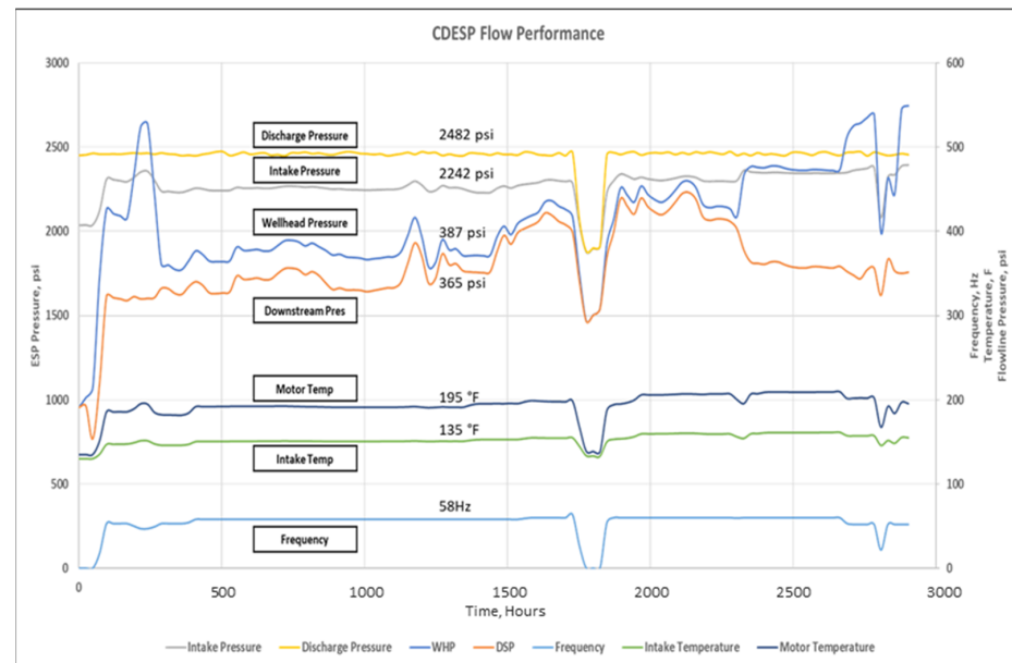
Figure 8. CDESP flow performance real-time parameters after redeployment; image displays the performance over almost 3000 h of operation.
