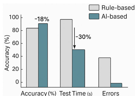
Figure 12. Comparative performance of rule-based and AI-based grading methods in terms of accuracy, test time, and error rate.
