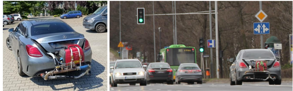
Figure 6. Vehicle undergoing RDE testing.
