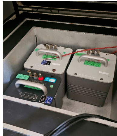
Figure 4. Standard inductors type GR1482-x (1 mH, 10 mH, and 1 H), placed in thermostatic chamber. Property of GUM.
