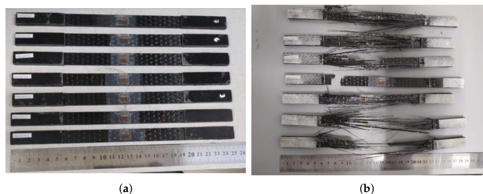
Figure 6. Tensile test specimens. (a) Before the test; (b) after the test. Test specimen numbers correspond to the results presented in Figure A5.
