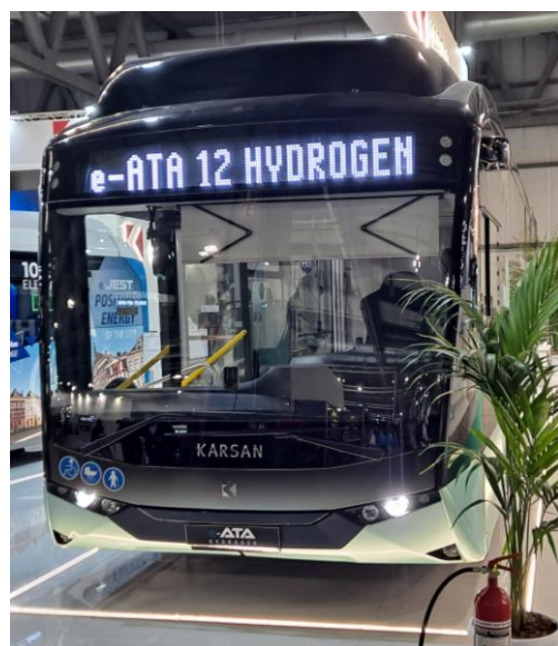
Figure 11. The hydrogen city bus with a range of 500 km.
