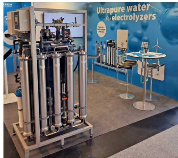
Figure 1. A commercial water preparation station for large-scale electrolytic processes, presented at the Hydrogen Technology Expo 2023 in Bremen, Germany.
