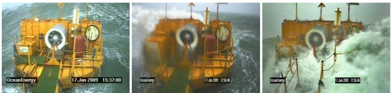
Figure 3. Large breaking waves interacting with the Ocean Energy Buoy whilst deployed at Galloway Bay, Ireland [16].
