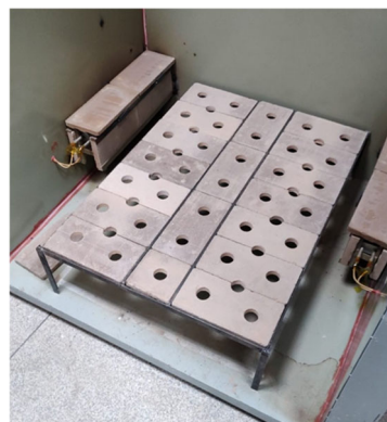
Figure 6. Cable separator structure.
