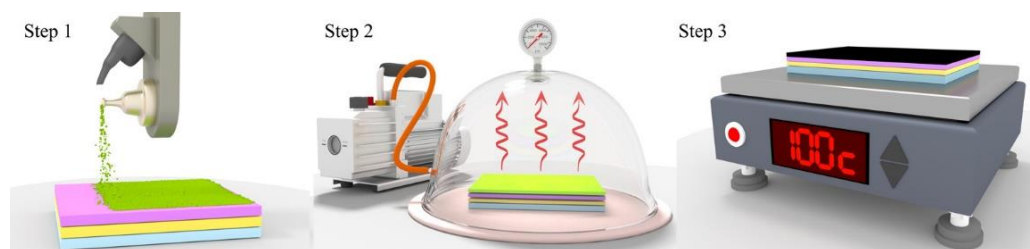
Figure 22. A schematic representation of the spray-deposition and VASP treatment methods designed for making high-quality perovskite films. ( Step 1 ), the spray head glides over the surface, depositing the precursor ink, which produces a wet coating. ( Step 2 ) the wet film is subjected to a partial vacuum to remove the DMF, leading to a partly crystallized layer. ( Step 3 ) the film is annealed at 100 °C. Reused with permission [108].
