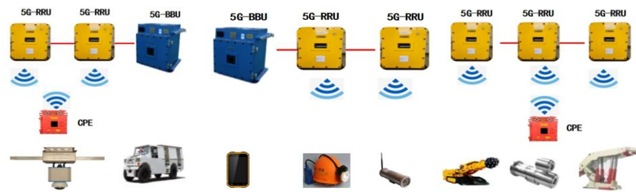
Figure 14. The electric control connection diagram with private 5G network access is applied to coal mines in China.
