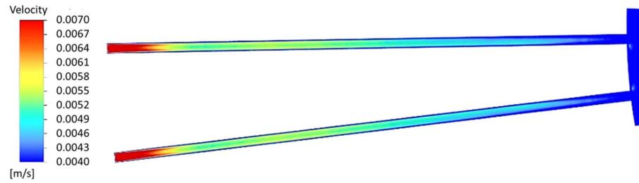
**Figure 7.** Oil velocity distribution inside fins' cross-section.
