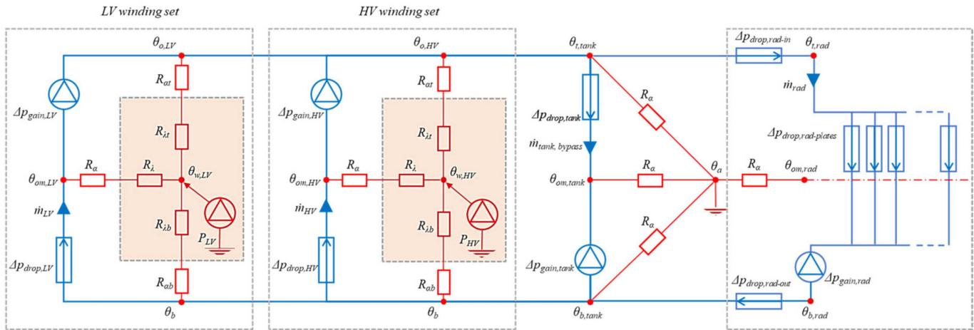
Figure 9. Thermal–hydraulic network of main windings, tank and radiator.
