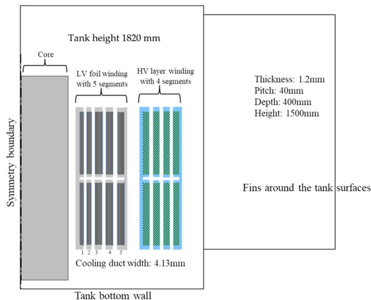
**Figure 2.** Layout of winding in the tank cross-section.
