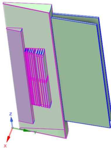
**Figure 3.** Simplified axisymmetric 3D model of the transformer.
