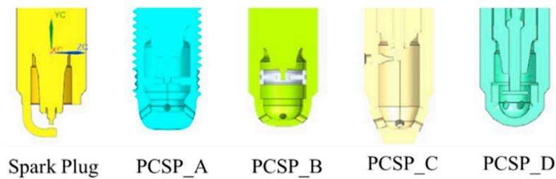
**Figure 4.** Electrode design of experimental spark plugs.
