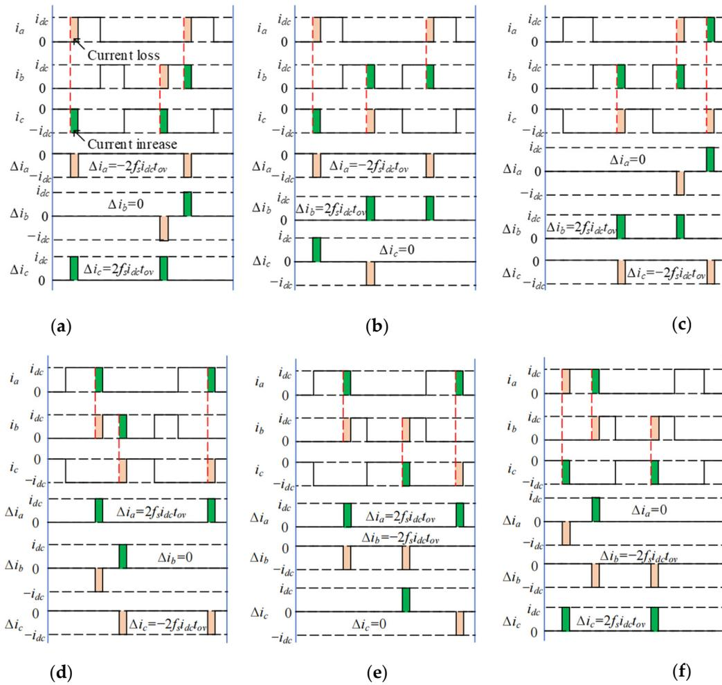
**Figure 7.** The diagrams of  $i_a$ ,  $i_b$ , and  $i_c$  with their error caused by the overlap time in sector II: (a)  $u_a > u_b > u_c$ ; (b)  $u_a > u_c > u_b$ ; (c)  $u_b > u_a > u_c$ ; (d)  $u_b > u_c > u_a$ ; (e)  $u_c > u_a > u_b$ ; (f)  $u_c > u_b > u_a$ .
