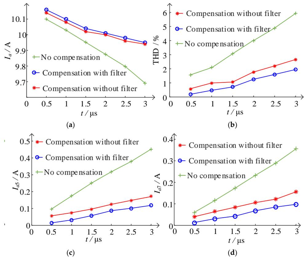
**Figure 20.** The comparison results of no compensation, compensation without discrete filter, and the proposed compensation under different overlap time: (a) fundamental amplitude; (b) THD; (c) amplitude of fifth harmonic; (d) amplitude of seventh harmonic.
