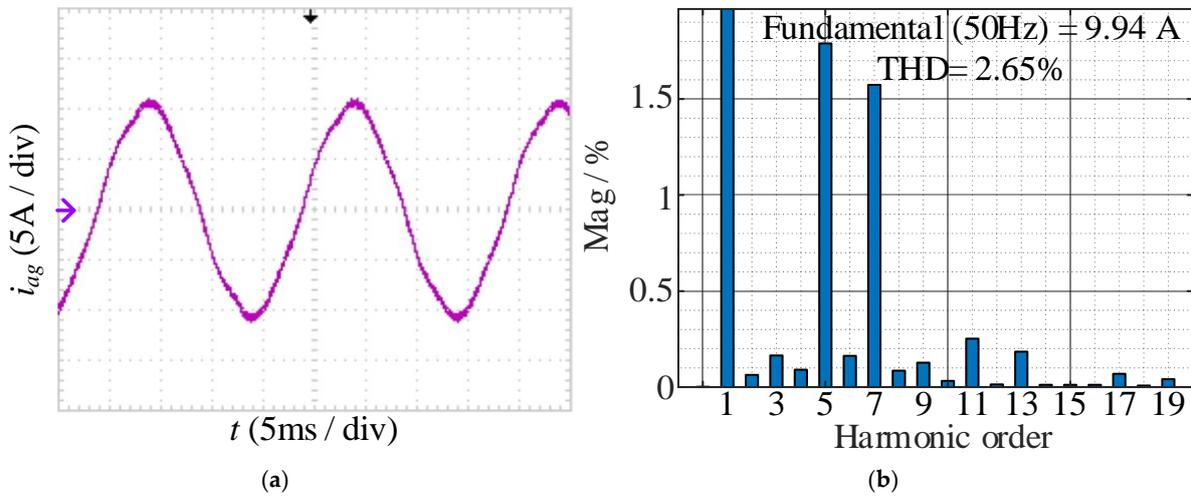
**Figure 19.** Experimental results with compensation and no discrete filter under  $t_{ov} = 3 \mu s$ : (a) waveform of  $i_{ag}$ ; (b) FFT results of  $i_{ag}$ . Purple arrow—the zero tick mark.
