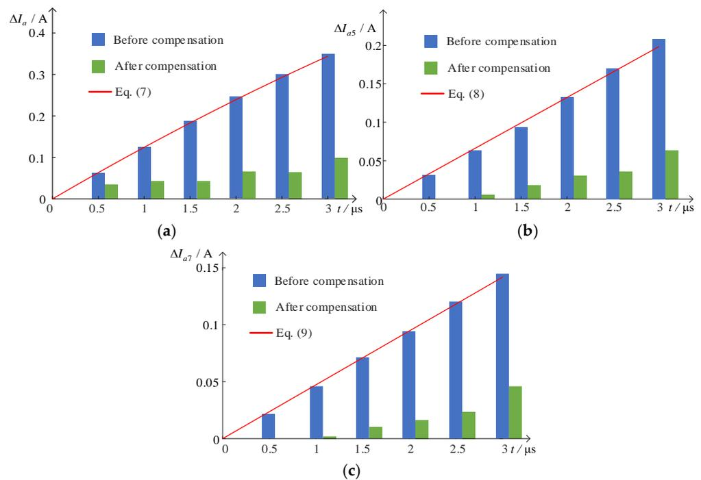
**Figure 14.** Comparison results of no compensation, proposed compensation, and derived harmonic expressions: (a)  $\Delta I_a$ ; (b)  $\Delta I_{a5}$ ; (c)  $\Delta I_{a7}$ .
