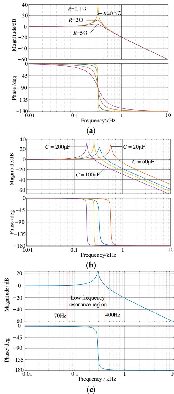
**Figure 9.** Bode plot of  $G_{i2ig}(s)$ : (a) different  $R$ ; (b) different  $C$ ; (c) parameters determined in this paper.
