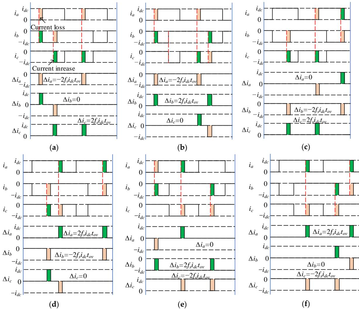
**Figure 6.** The diagrams of  $i_a$ ,  $i_b$ , and  $i_c$  with their error caused by the overlap time in sector I: (a)  $u_a > u_b > u_c$ ; (b)  $u_a > u_c > u_b$ ; (c)  $u_b > u_a > u_c$ ; (d)  $u_b > u_c > u_a$ ; (e)  $u_c > u_a > u_b$ ; (f)  $u_c > u_b > u_a$ .
