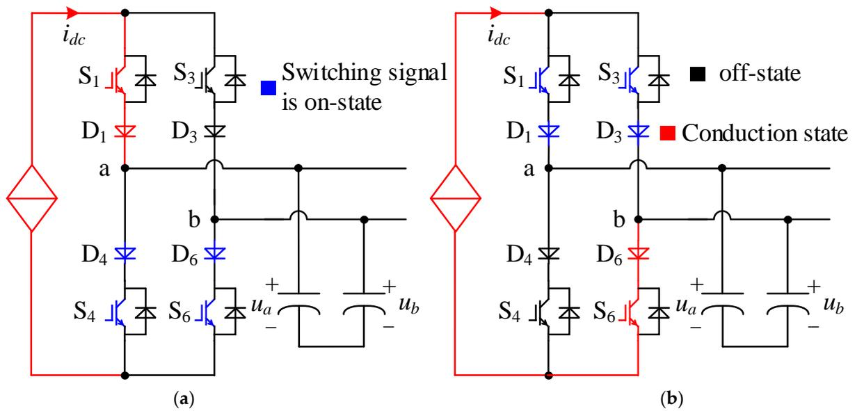
**Figure 5.** Equivalent circuit during the overlap time: (a) commutation from  $I_7$  to  $I_1$ ; (b) commutation from  $I_8$  to  $I_1$ .
