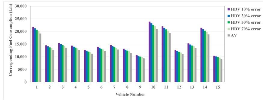
**Figure 7.** Aggregate fuel consumption by driver behavior for upper limits of platooning.
