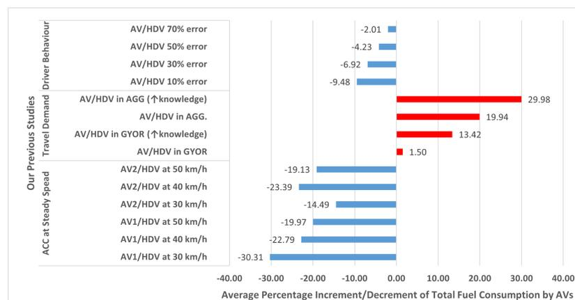
Figure 27. Percentage of total fuel consumption of AVs to HDVs at upper energy savings limits.
