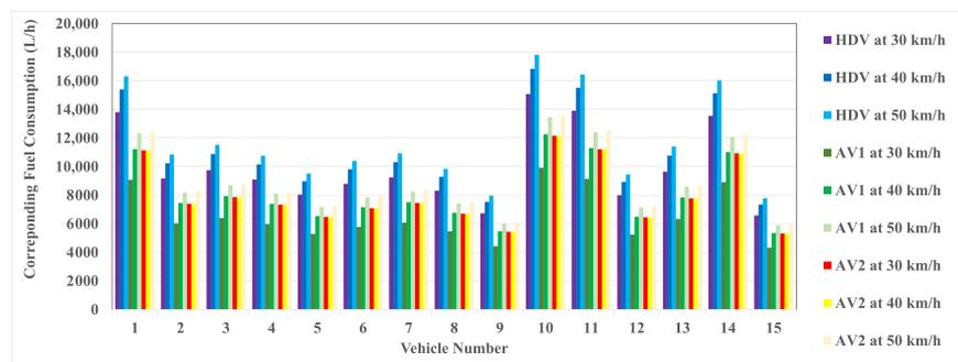
Figure 24. Aggregate fuel consumption by ACC at steady speeds for upper limits of powertrain.
