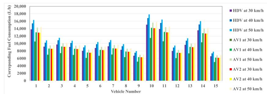
**Figure 18.** Aggregate fuel consumption by ACC at steady speeds lower limits of car-following.
