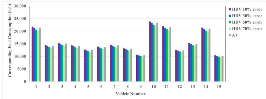
Figure 4. Aggregate fuel consumption by driver behavior for lower limits of powertrain.
