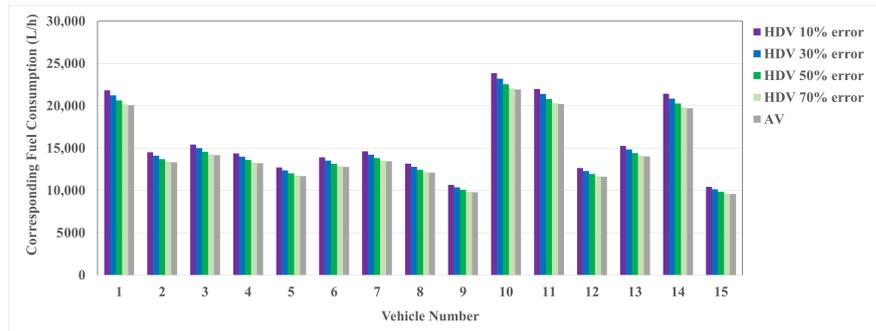
Figure 6. Aggregate fuel consumption by driver behavior for upper limits of car-following.
