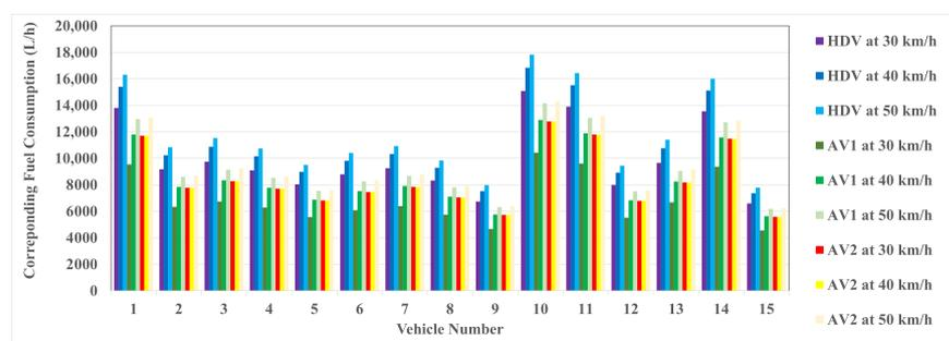
Figure 25. Aggregate fuel consumption by ACC at steady speeds for upper limits of intersection control.
