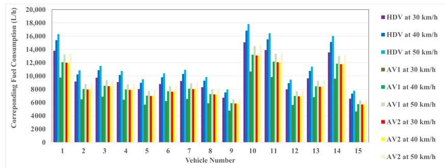
Figure 22. Aggregate fuel consumption by ACC at steady speeds for upper limits of car-following.
