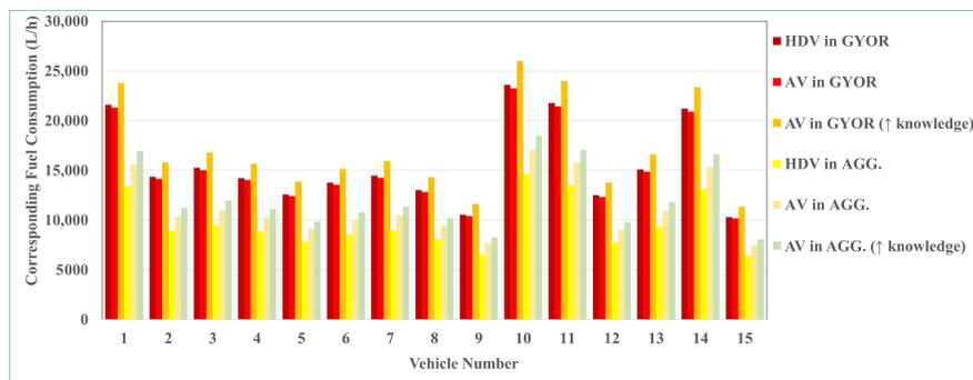
Figure 15. Aggregate fuel consumption by travel demand for upper limits of platooning.
