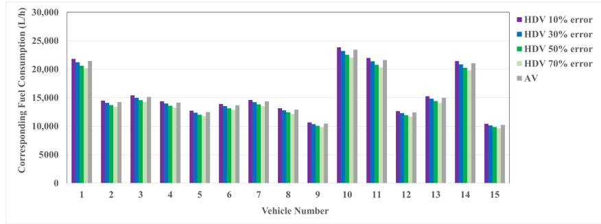
Figure 3. Aggregate fuel consumption by driver behavior for lower limits of platooning.
