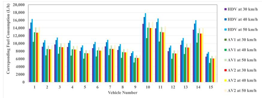
Figure 20. Aggregate fuel consumption by ACC at steady speeds for lower limits of powertrain.
