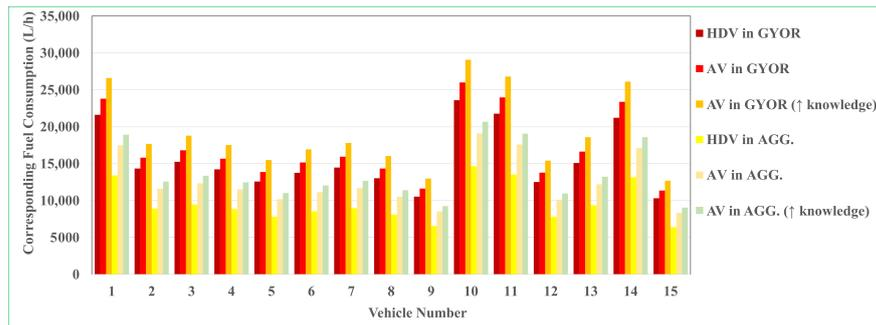
Figure 11. Aggregate fuel consumption by travel demand for lower limits of platooning.
