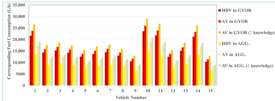
Figure 12. Aggregate fuel consumption by travel demand for lower limits of powertrain.
