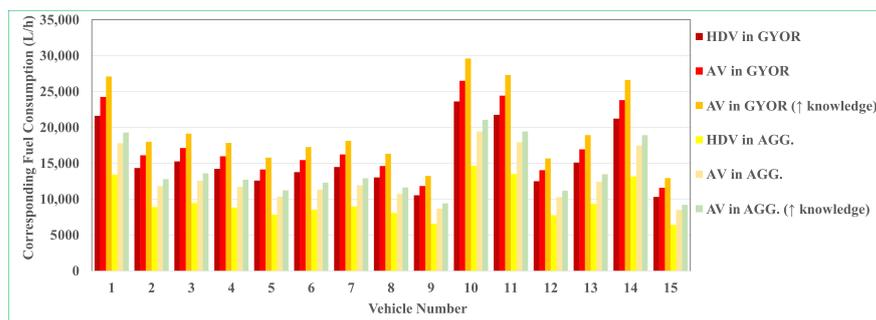
Figure 13. Aggregate fuel consumption by travel demand for lower limits of intersection control.
