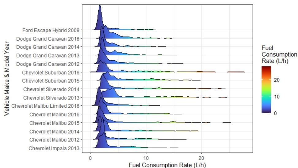
**Figure 1.** Tested vehicles and corresponding fuel consumption rates, based on [22].
