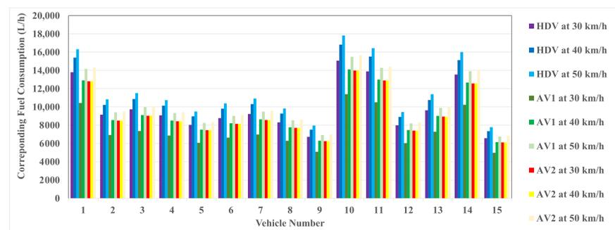
**Figure 19.** Aggregate fuel consumption by ACC at steady speeds lower limits of platooning.
