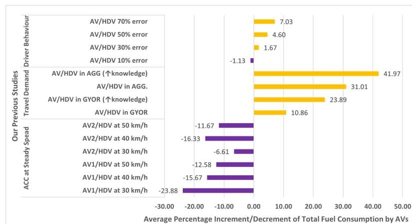
Figure 26. Percentage of total fuel consumption of AVs to HDVs at lower energy savings limits.
