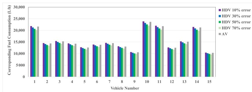
**Figure 2.** Aggregate fuel consumption by driver behavior for lower limits of car-following.
