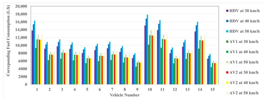
Figure 23. Aggregate fuel consumption by ACC at steady speeds for upper limits of platooning.
