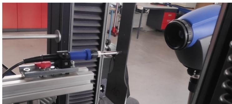
**Figure 7.** The stand for identification of heat flux parameters with a thermographic camera.
