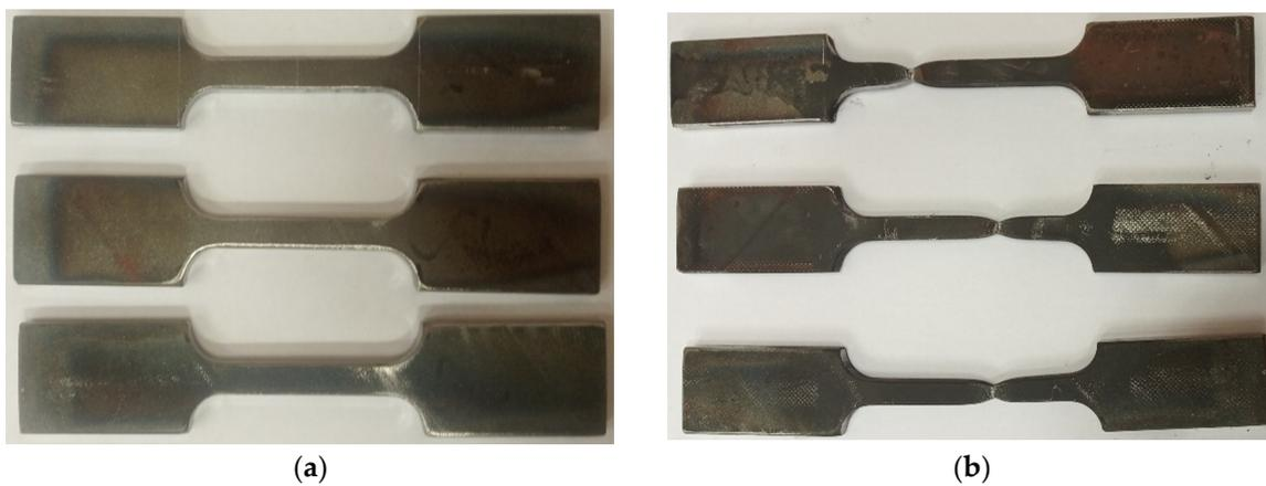
**Figure 2.** The specimens (a) before and (b) after static tensile tests.
