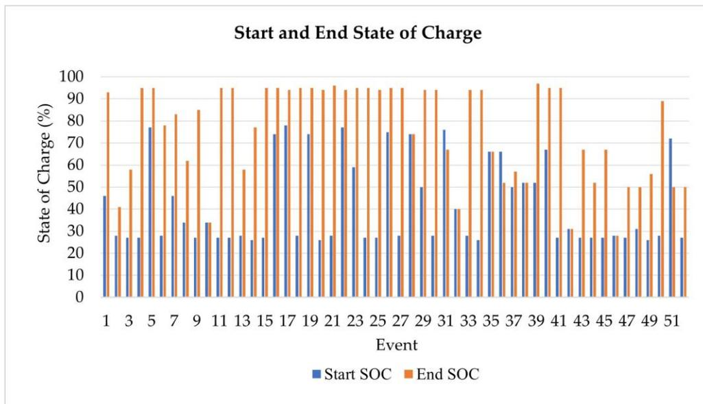
(a) Start and end SOC of the events registered by the charger installed at CEH
