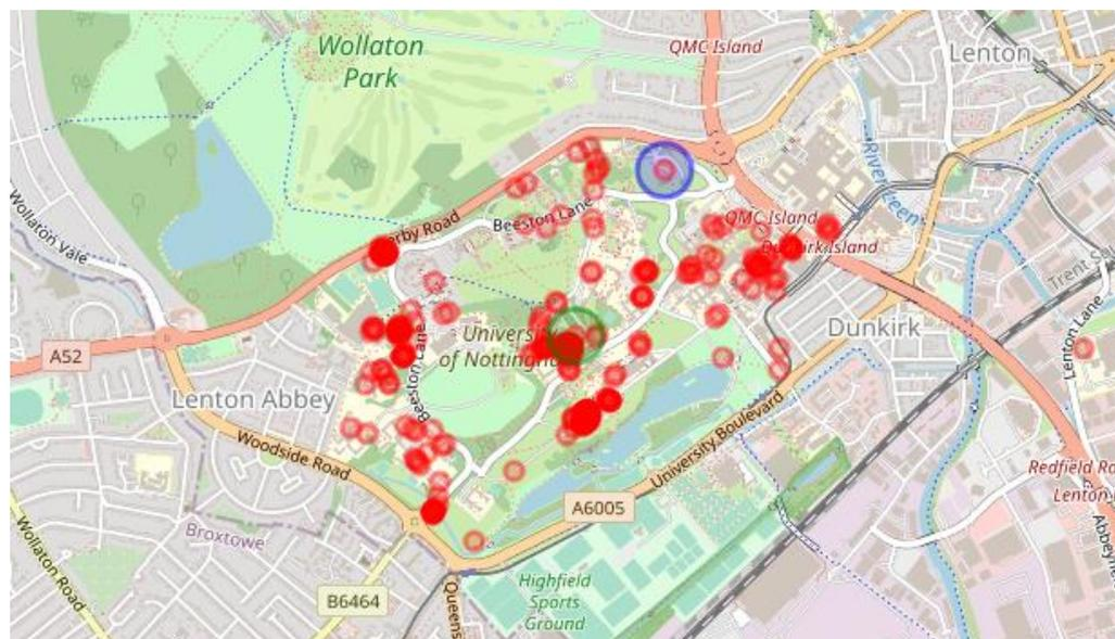
**Figure 25.** Locations of the vehicle with standing time more than 30 min. In blue is marked the location of the Creative Energy Homes charger, and in green the location of the Hallward Library charger. The red colour represents the places where the vehicles remain idle.
