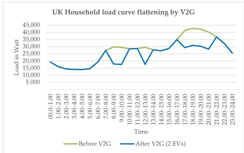
Figure 28. UK Household-Load-Curve Flattening by V2G.
