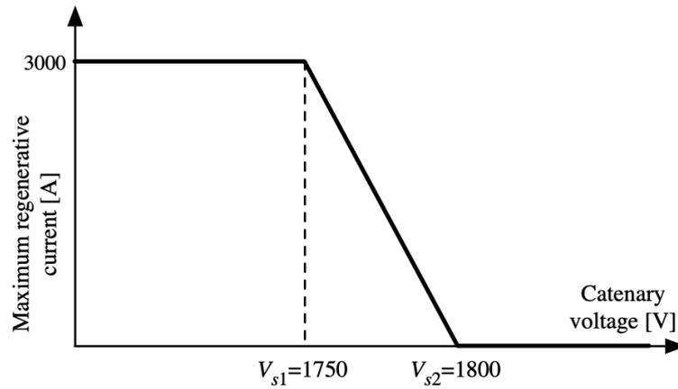
Figure 5. Regenerative Current Output Control.
