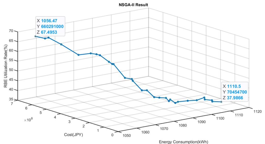
**Figure 13.** Case D: Cost Energy Regenerative Braking Energy Utilization rate.
