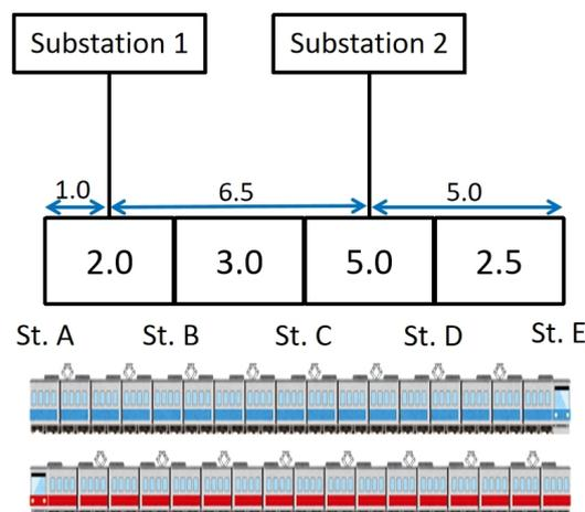
Figure 6. Topology of the Railway without ESS.
