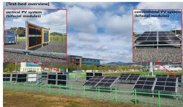
**Figure 2.** Testbed placement and data analysis targets (conventional PV system and vertical PV system with bifacial modules).
