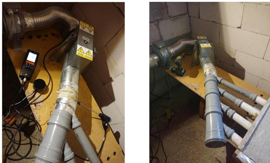
Figure 6. Heating group: fan, electric heater, and connected temperature sensor (on the left); flow distribution manifold (on the right) (before insulation).
