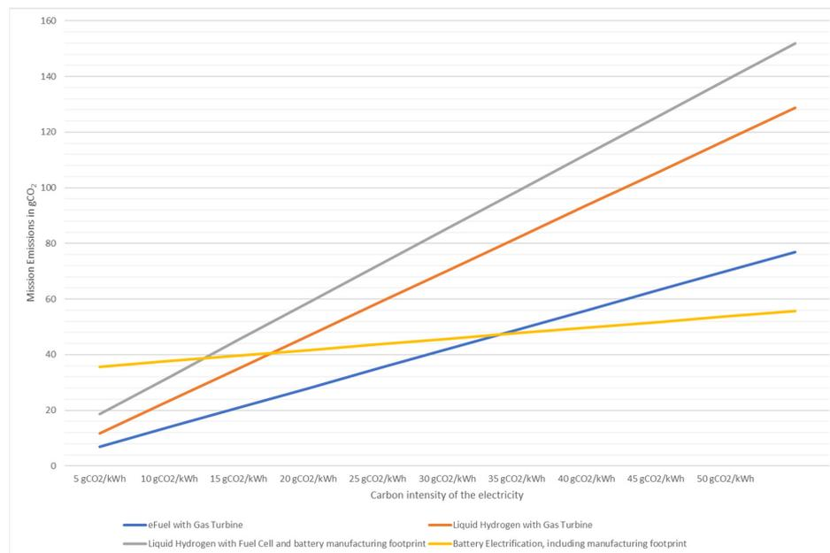
**Figure 6.** CO<sub>2</sub> emissions calculated for each energy vector with an electricity CI from 5 to 50 gCO<sub>2</sub>/kWh.
