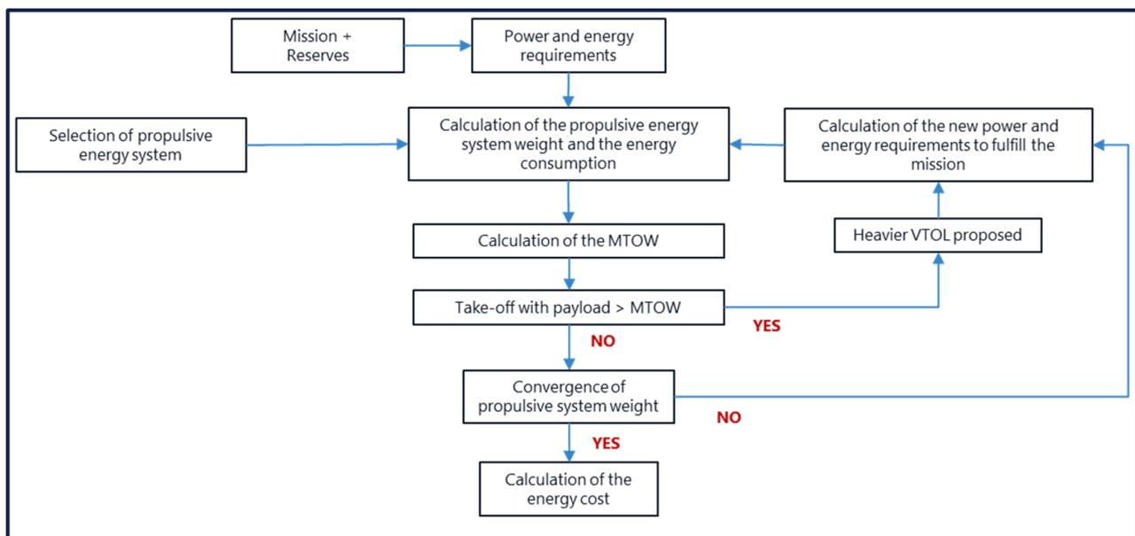
**Figure 4.** Design step for calculation.
