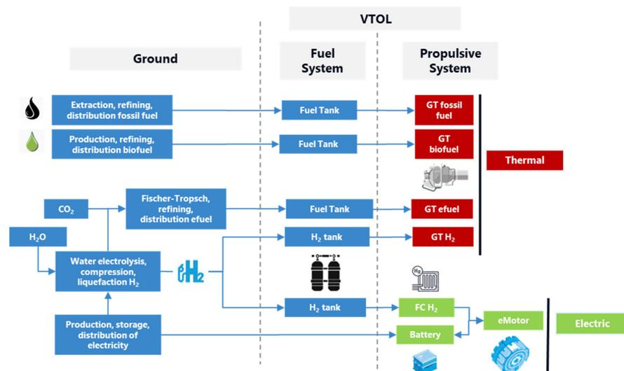
**Figure 1.** Energy carriers applied to VTOL with the associated propulsive architecture.
