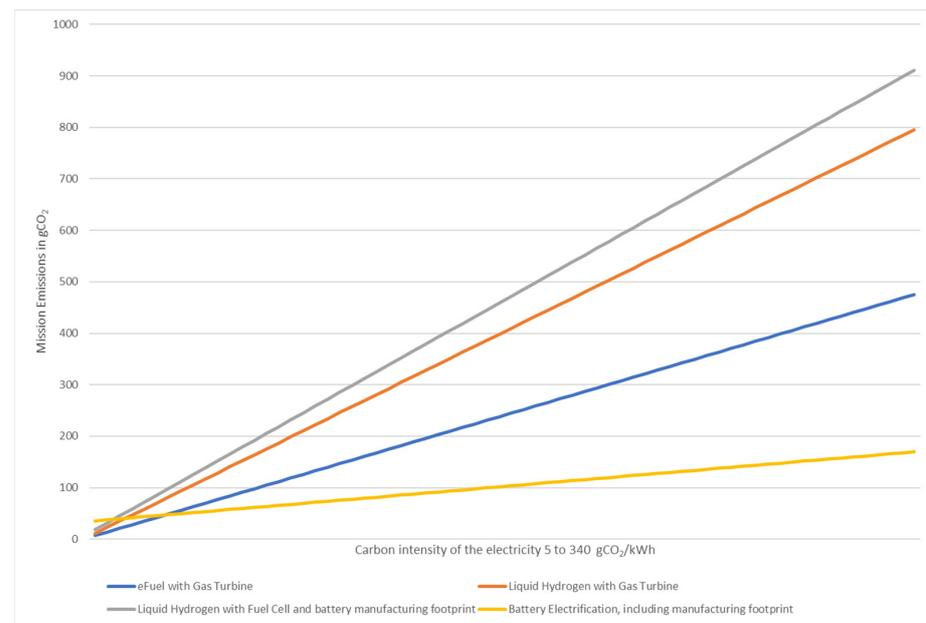
**Figure 5.** CO<sub>2</sub> emissions calculated for each energy carrier with an electricity CI from 5 to 340 gCO<sub>2</sub>/kWh.
