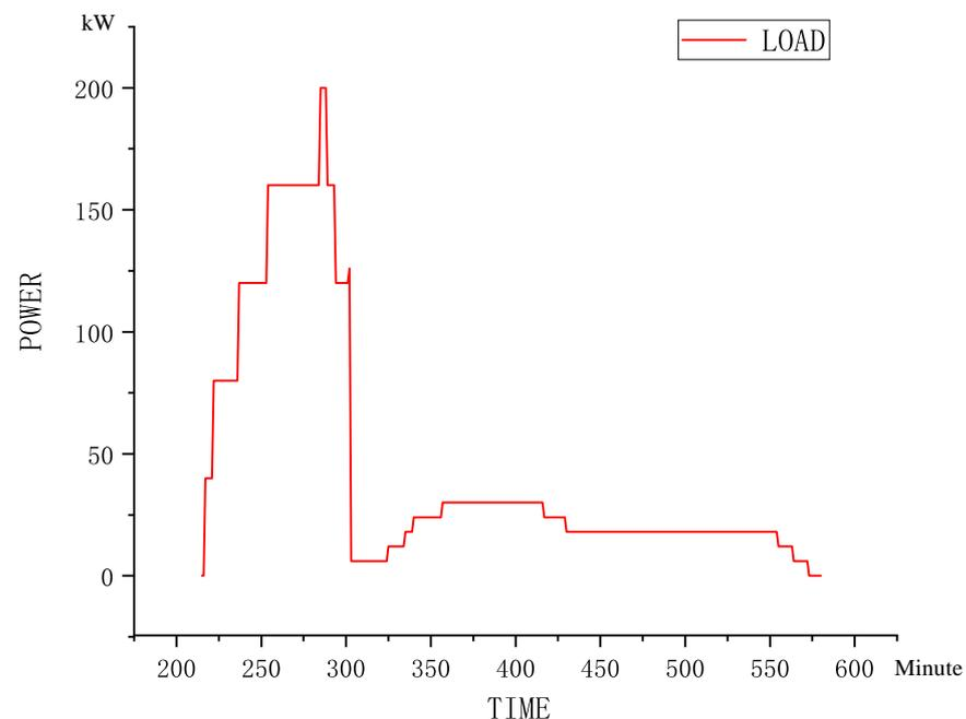
**Figure 7.** The charging load fluctuation of ETs for the ETPSS–ER system.
