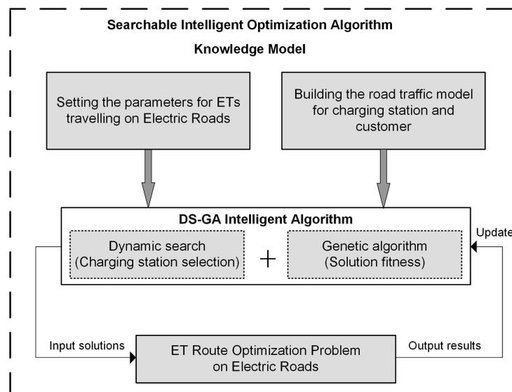
**Figure 2.** Structure of DS–GA optimization algorithm for the ET routing problem.
