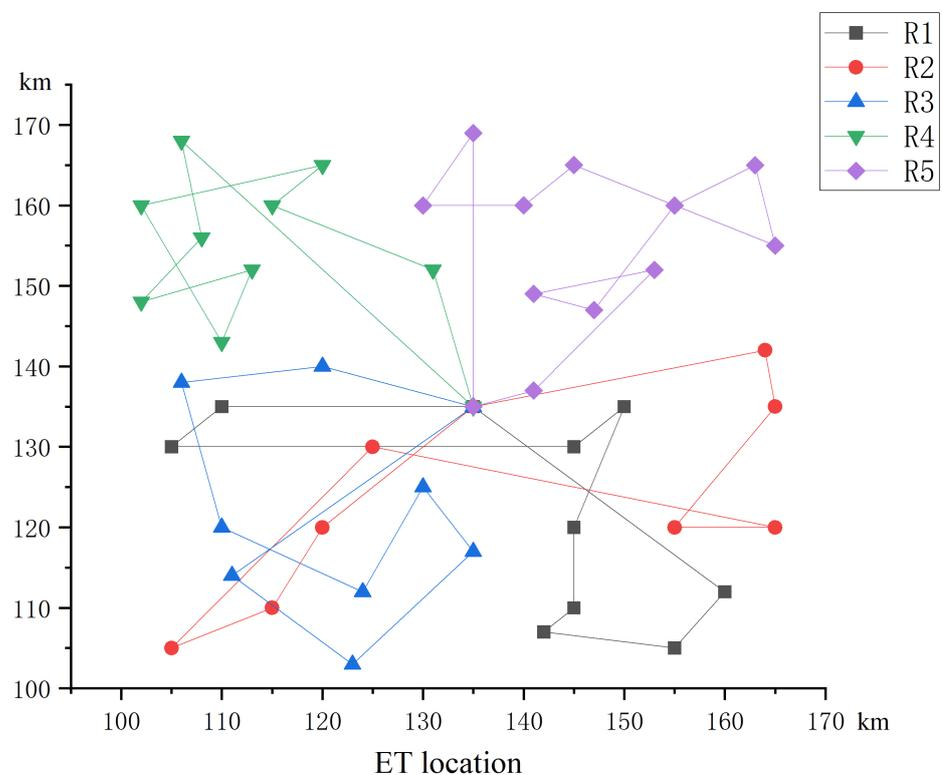
**Figure 6.** The optimal routes of ETs traveling on electric roads.
