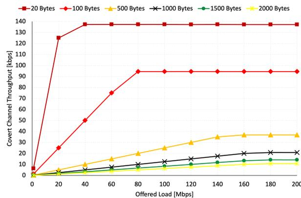
**Figure 5.** Covert channel throughput vs. offered load for different payload sizes and 1 STA.
