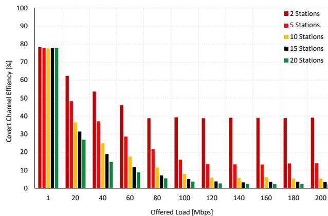
Figure 13. Covert channel efficiency vs. regular stations offered load.
