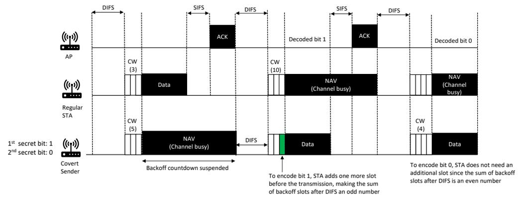
Figure 3. Covert Channel Operation.
