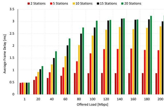
Figure 11. Covert channel delay vs. regular stations offered load.
