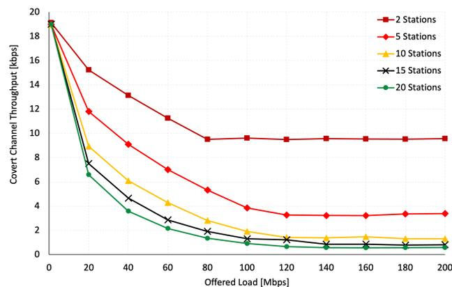
**Figure 10.** Covert channel throughput vs. regular stations offered load.
