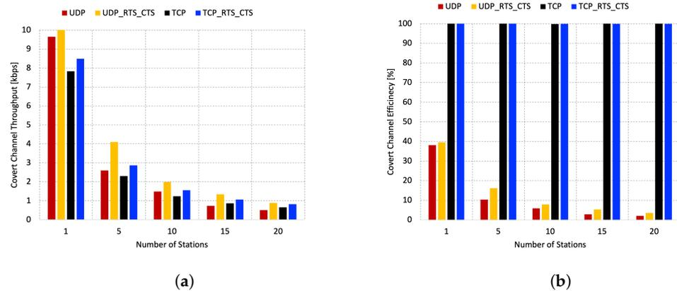
Figure 6. Covert channel throughput and efficiency analysis. (a) Throughput; (b) Efficiency.
