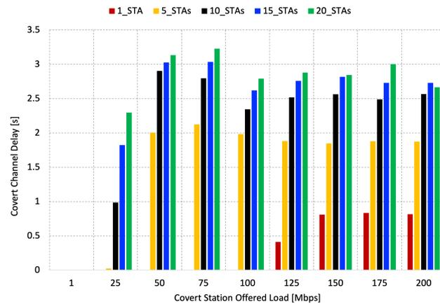
Figure 16. Delay of the covert channel for UDP Traffic.
