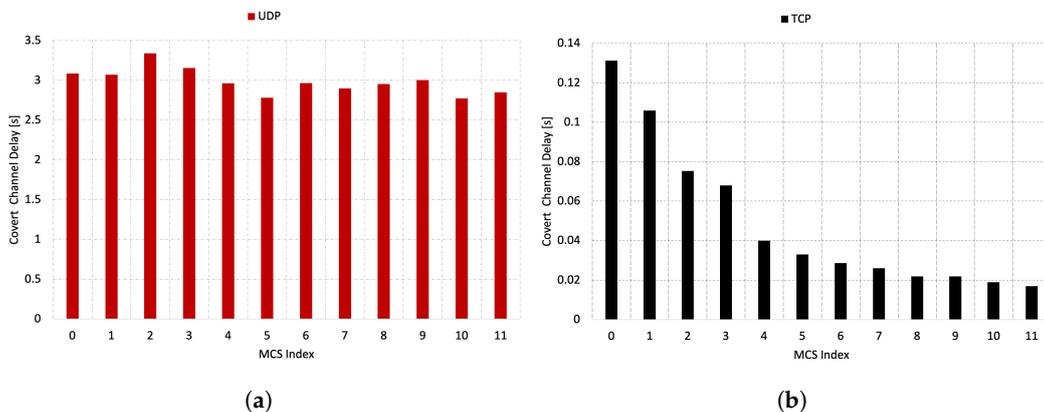
Figure 9. Delay of the covert channel in relation to the MCS Index. (a) UDP Traffic; (b) TCP Traffic.
