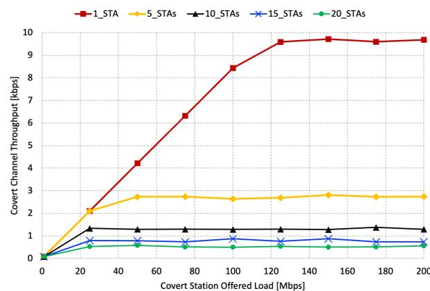
Figure 14. Throughput of the covert channel for UDP Traffic.
