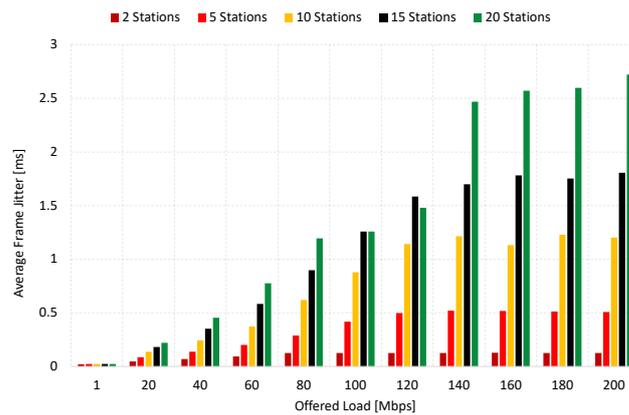
Figure 12. Covert channel average jitter vs. regular stations offered load.
