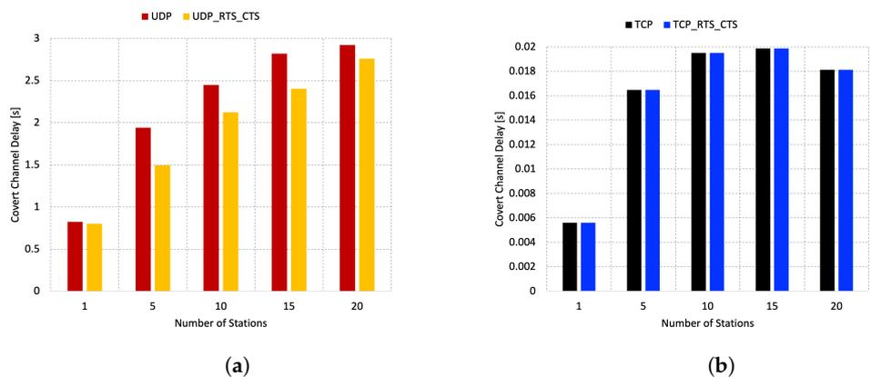
Figure 7. Covert channel delay analysis in relation to the number of stations. (a) UDP Traffic; (b) TCP Traffic.
