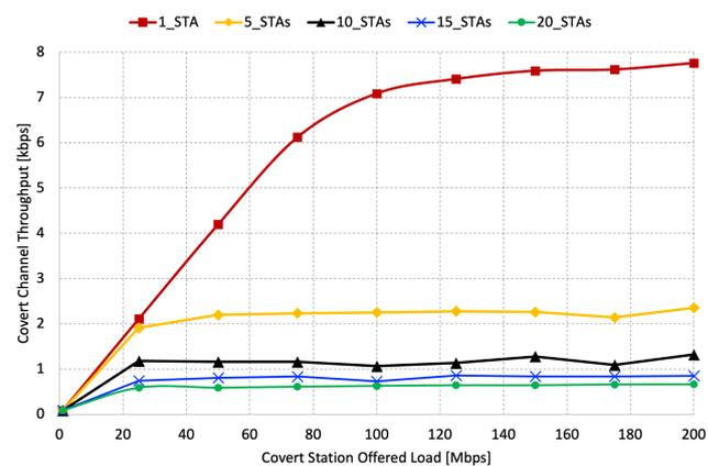
Figure 15. Throughput of the covert channel for TCP Traffic.
