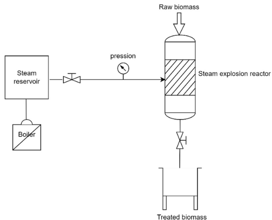
**Figure 2.** Schematic diagram of steam explosion process.
