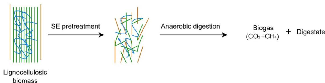
**Figure 1.** Lignocellulosic biomass valorisation by technological coupling of steam explosion and anaerobic digestion.
