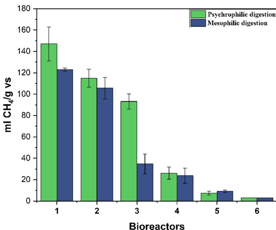
**Figure 5.** Cumulative methane production (mL/g vs). Bioreactor 1: SE with a lower concentration of the acid catalyst,  $S/I = 1/2$ ; Reactor 2: SE with higher conditions, SF #3,  $S/I = 1/2$ ; Bioreactor 3: SE a higher concentration of the acid catalyst,  $S/I = 1/2$ ; Bioreactor 4: SE with higher conditions,  $S/I = 1/1$ ; Bioreactor 5: SE with lower conditions,  $S/I = 1/2$ ; Bioreactor 6: Raw biomass (without SE treatment).
