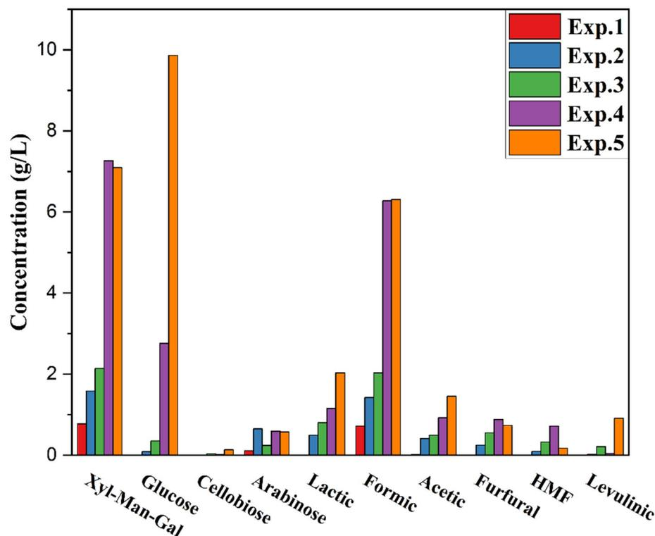
**Figure 4.** The HPLC Quantification of Sugars and Degradation Compounds under Steam Explosion (SE) Conditions.
