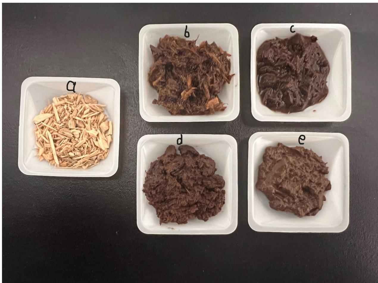
**Figure 3.** SE effect on wood chips morphology. (a) Untreated biomass, (b) SE with medium conditions of T and P, (c) SE with high conditions of T and P, (d) SE with a low concentration of an acid catalyst, (e) SE with a high concentration of an acid catalyst.
