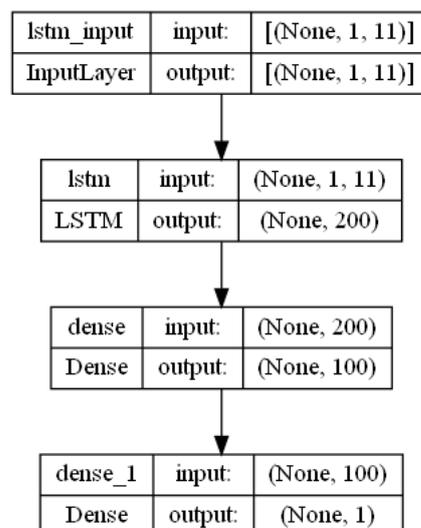
Figure 1. Multi-LSTM DNN model architecture.
