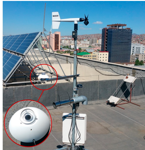
Figure 4. Weather station located at the Ulaanbaatar site. The pyranometer is zoomed in for a better view.
