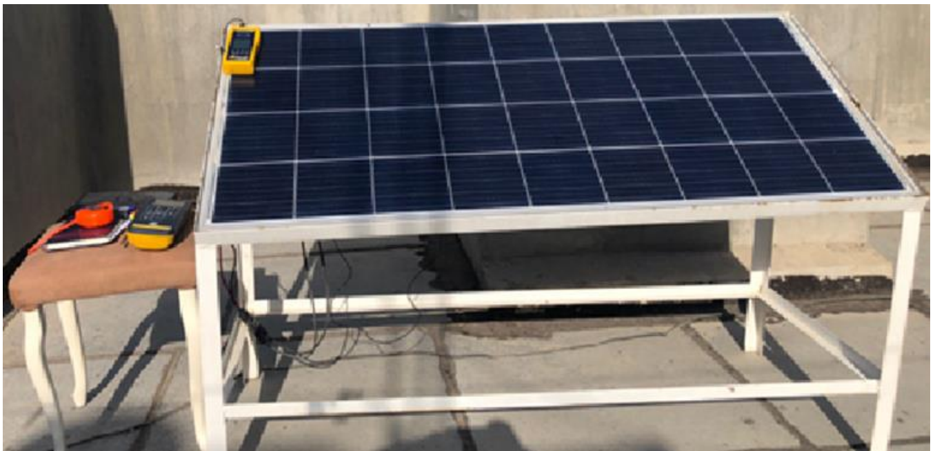
Figure 3. Setup of PV module with measuring devices.
