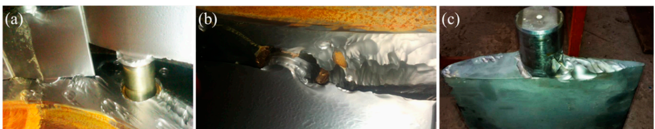
Figure 1. Erosion due to secondary flows at the clearance gap of GVs: (a) toward the bottom facing plate, (b) toward the upper facing plate, and (c) eroded GV toward the bottom end.
