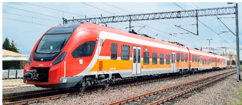
Figure 3. Three car body diesel–electric multiple unit.
