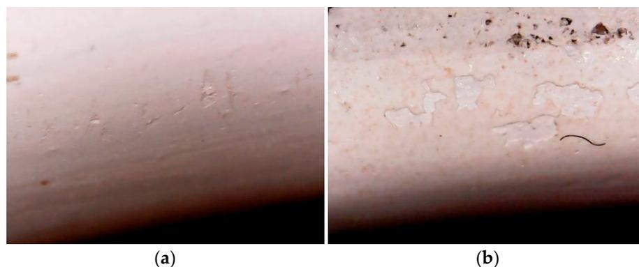
**Figure 19.** Erosion topography on leading edge of the blade 0.3R–0.7R: (a) Particle size of 0–1 mm; (b) Particle size of 1–2 mm.
