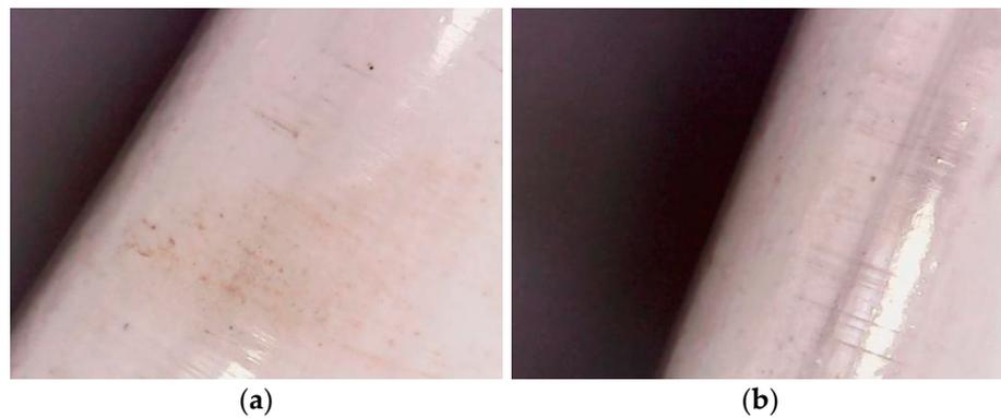
**Figure 24.** Erosion topography on trailing edge of the blade root-0.3R: (a) Particle size of 0–1 mm; (b) Particle size of 1–2 mm.
