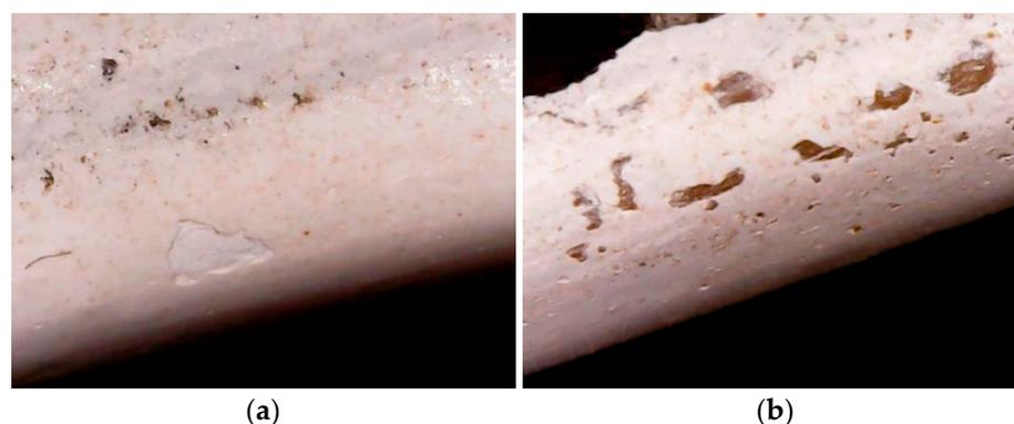
**Figure 20.** Erosion topography on leading edge of the 0.7R-blade tip: (a) Particle size of 0–1 mm; (b) Particle size of 1–2 mm.
