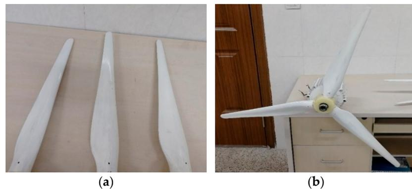
**Figure 11.** The miniature model of 1.5 MW horizontal axis wind turbine: (a) Blade; (b) Wind rotor.
