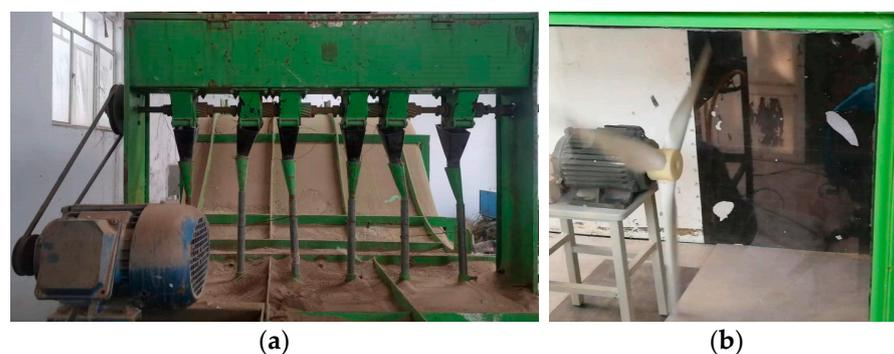
**Figure 15.** Wind-sand erosion test on wind turbine blades: (a) Sand conveyor; (b) Rotating wind rotor.
