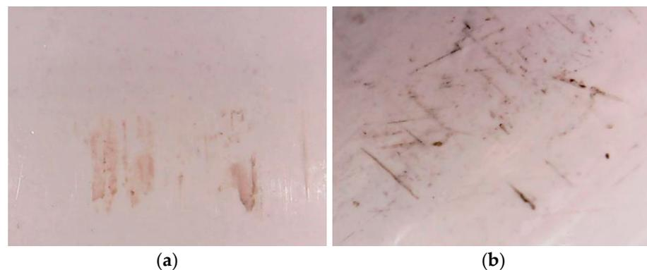
**Figure 22.** Erosion topography on windward side of the blade 0.3R–0.7R: (a) Particle size of 0–1 mm; (b) Particle size of 1–2 mm.
