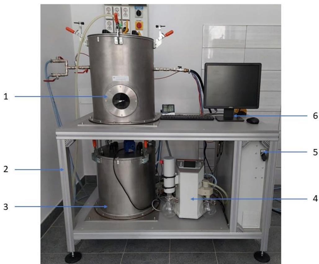
**Figure 1.** The scheme of the experimental test stand marked with the most essential elements: 1—reaction chamber; 2—aluminum frame; 3—evaporator chamber; 4—laboratory vacuum system; 5—data acquisition and control system; 6—PC.
