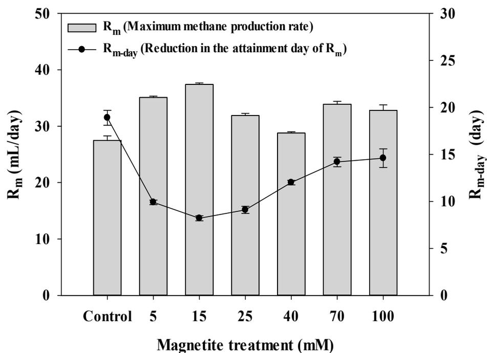
**Figure 5.**  $R_m$  and  $R_{m-day}$  by concentration according to the addition of magnetite ( $B_u$  mean of maximum methane production rate and  $R_{m-day}$  mean of reduction in the attainment day of  $R_m$ ).
