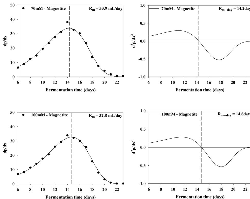
**Figure 3.** Analysis of maximum methane production rate and attainment day by the 1st and 2nd derivative from the cumulative methane production curve of  $\text{Fe}_3\text{O}_4$  addition.
