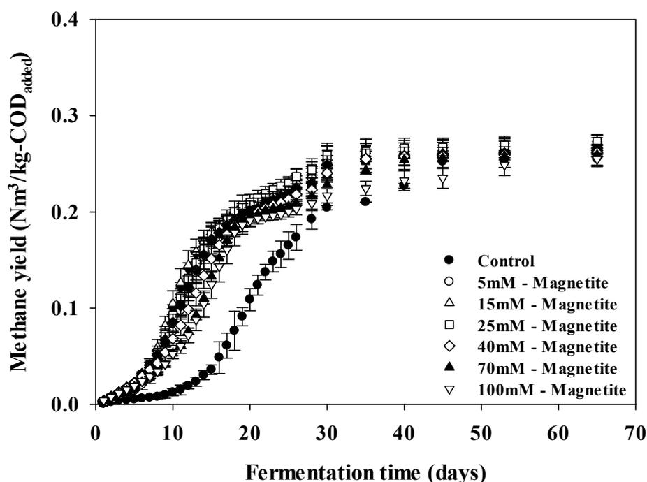
Figure 1. Methane yield curve by the addition of magnetite.
