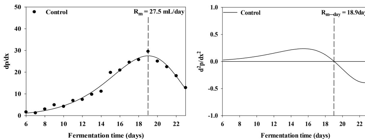
**Figure 2.** Analysis of maximum methane production rate and attainment day by the 1st and 2nd derivative from the cumulative methane production curve of control.
