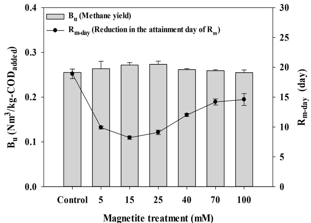
**Figure 4.**  $B_u$  and  $R_{m\text{-day}}$  by concentration according to the addition of magnetite ( $B_u$  mean of methane yield and  $R_{m\text{-day}}$  mean of reduction in the attainment day of  $R_m$ ).
