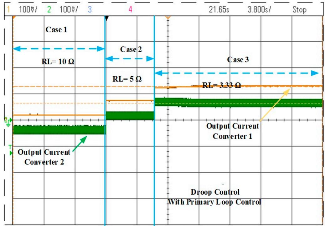
Figure 16. The output current of two converters at droop gain with primary control during load changes of 10 to 5 and 3.33 and input voltage changes.
