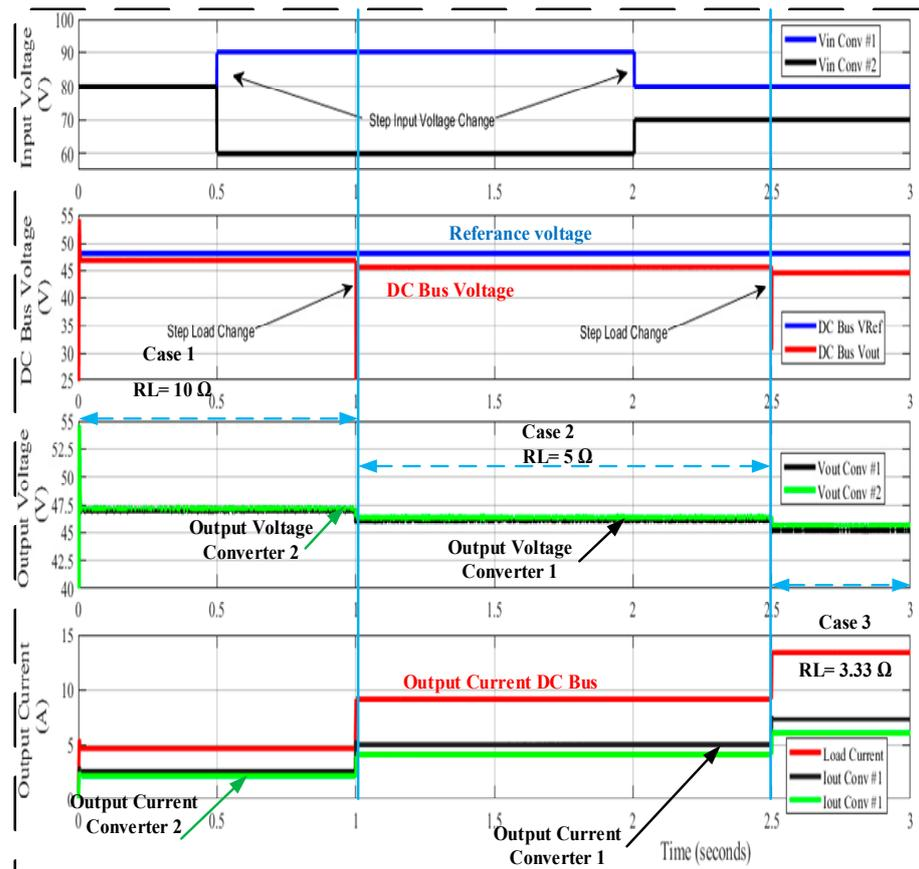
Figure 12. The transient response for Droop gain with primary control MATLAB/SIMULINK with a step load change from 10 Ω to 5 Ω and 3.33 Ω and step change in the input voltage.
