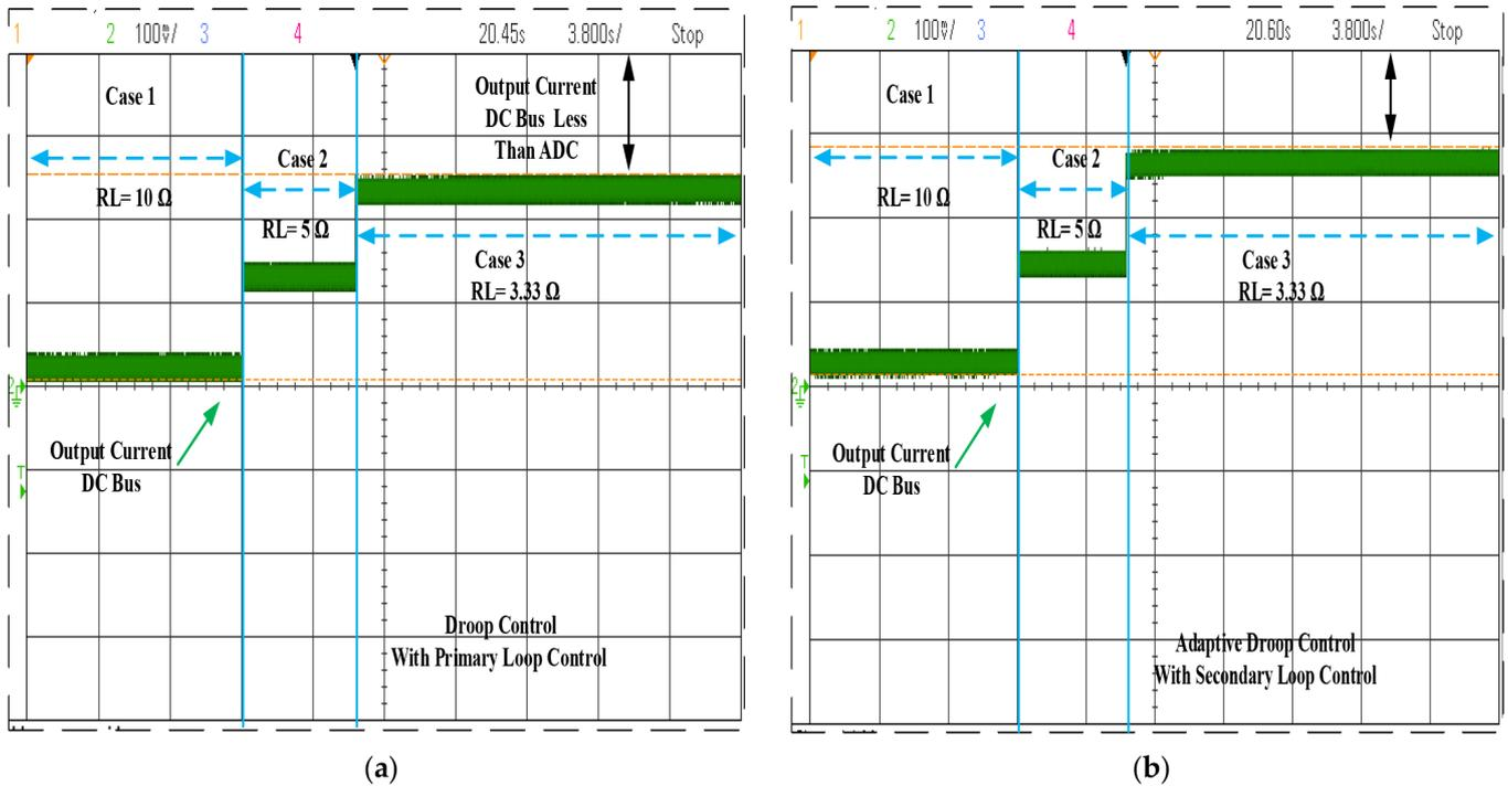
Figure 20. Comparison between current DC bus at (a) Droop gain with primary control, (b) Adaptive droop gain with secondary control during load changes of 10 to 5 and 3.33 and input voltage changes.
