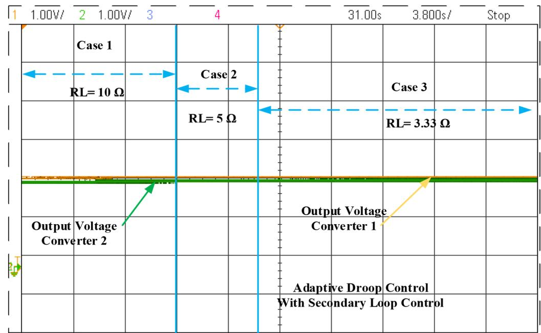
Figure 15. The output voltage of adaptive droop gain with secondary control during load changes of 10 to 5 and 3.33 and input voltage changes.
