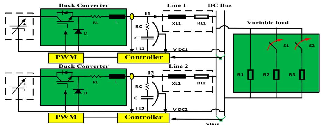
**Figure 2.** DC-DC buck converter configuration scheme.
