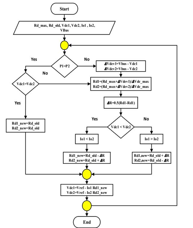
Figure 8. Flowchart for droop control technique submitted.
