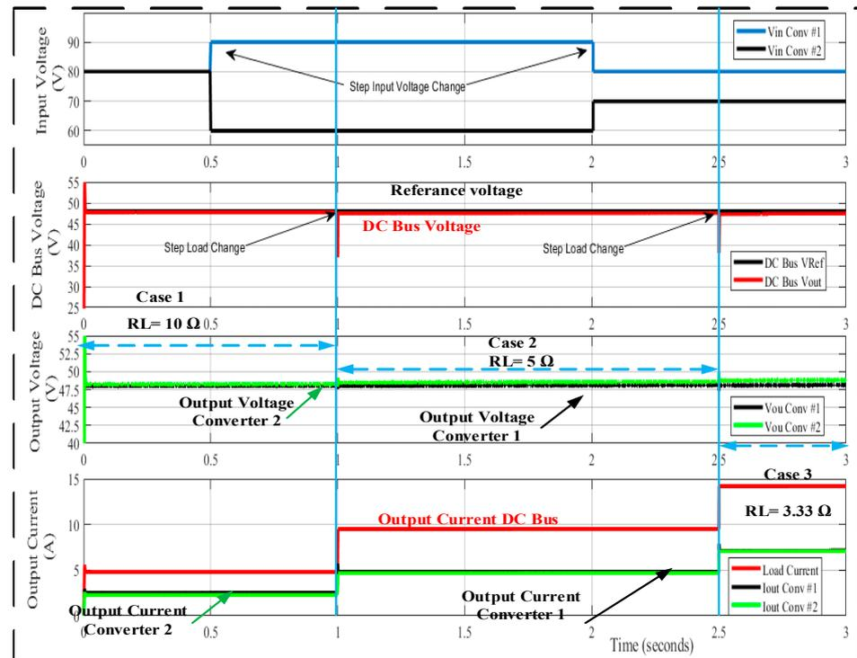
Figure 13. The transient response Adaptive droop gain with secondary control MATLAB/SIMULINK with a step load change from 10 Ω to 5 Ω and 3.33 Ω and step change in the input voltage.
