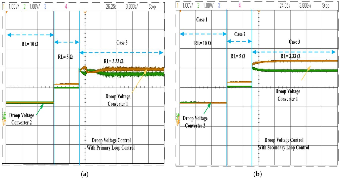
**Figure 11.** Comparison between Droop Voltage at (a) Droop Voltage with primary control, (b) Droop Voltage with secondary control during load changes of 10 to 5 and 3.33 and input voltage changes.
