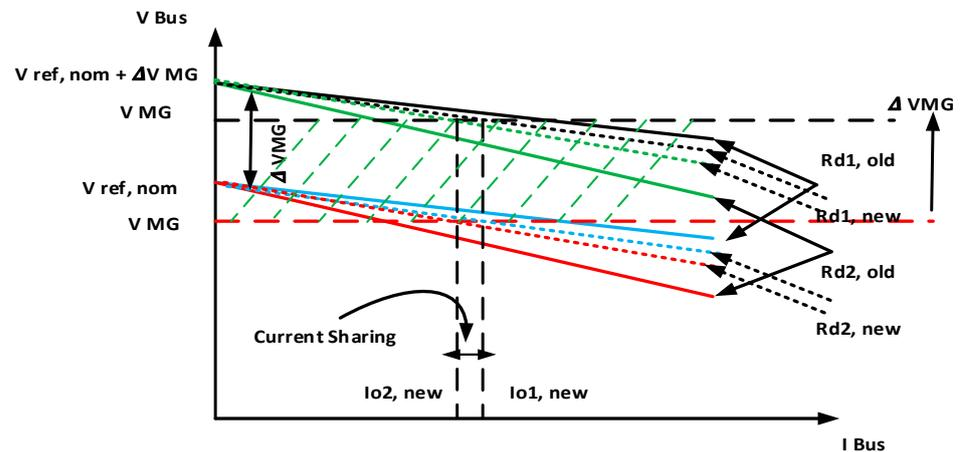
Figure 9. The bus voltage between the two DG units has been restored.
