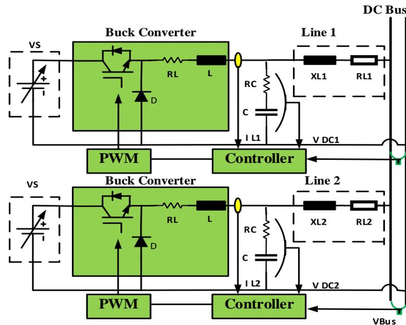
Figure 1. Power sources in the DC-MG configuration can be interconnected.
