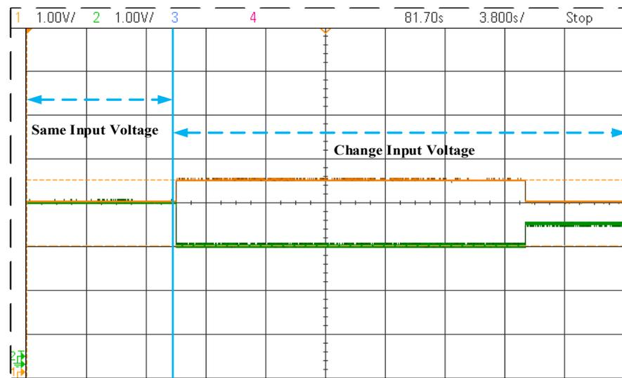
Figure 10. Change the input voltage of two buck converters.
