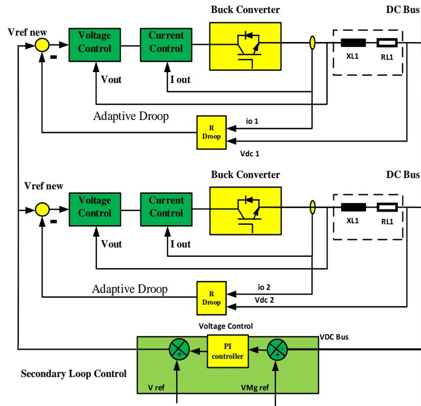
Figure 6. Parallel buck converter control schematic with adaptive droop control.
