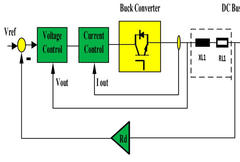
Figure 4. Traditional droop control for distributed resource DC microgrids.
