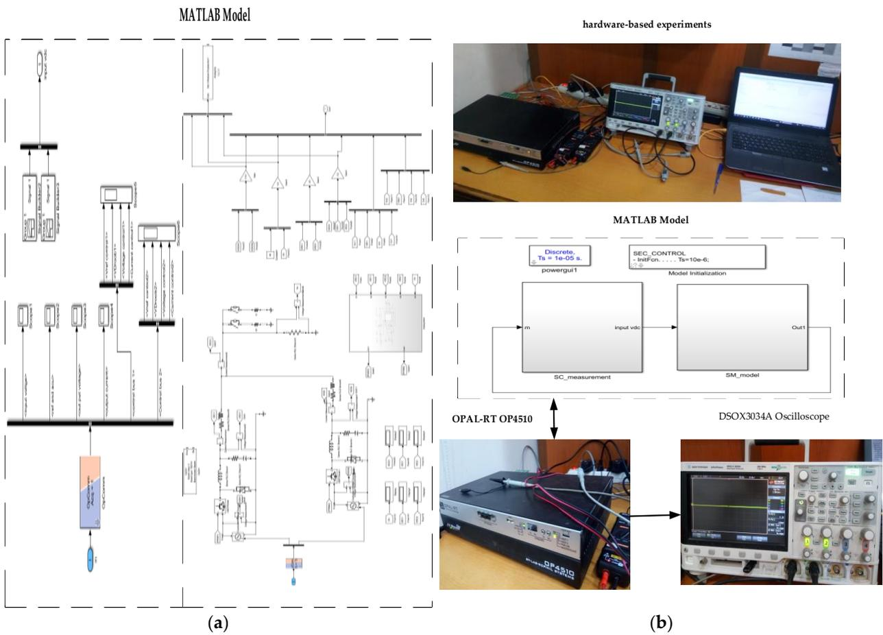
Figure 7. (a) Simulation model. (b) Real-Time OPAL-RT OP4510.
