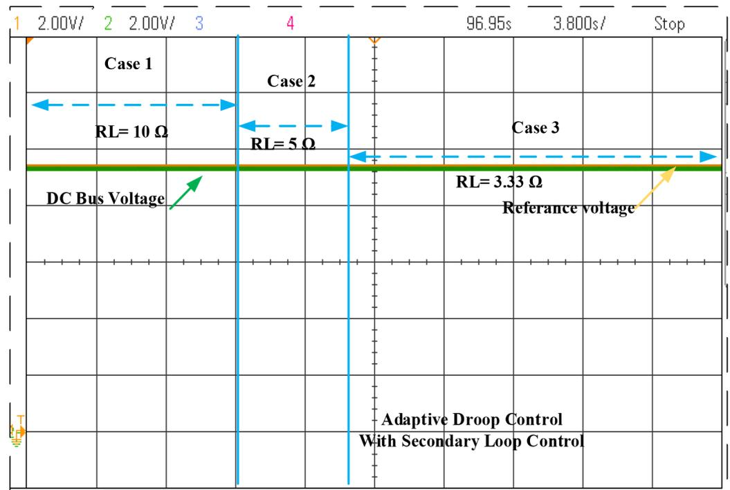
Figure 19. Bus voltage at adaptive droop gain with secondary control during load changes of 10 to 5 and 3.33 and input voltage changes.
