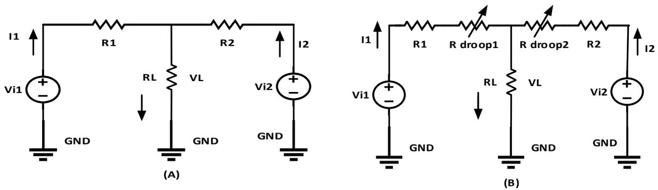
**Figure 3.** (A) Equivalent DC-DC circuit. (B) Equivalent DC-DC circuit with R droop.
