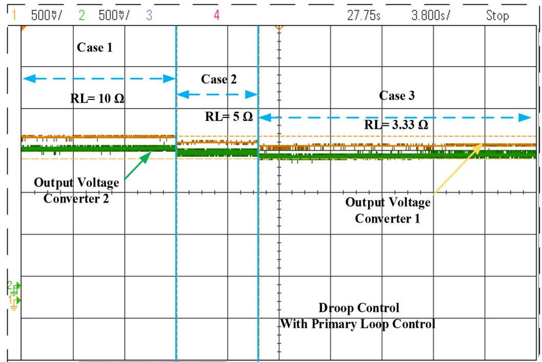
Figure 14. Output voltage of droop gain with primary control, during load changes of 10 to 5 and 3.33 and input voltage changes.
