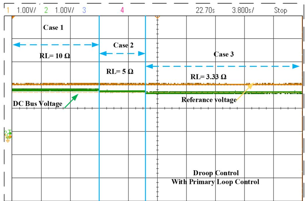
**Figure 18.** Bus voltage at droop gain with primary control, during load changes of 10 to 5 and 3.33 and input voltage changes.
