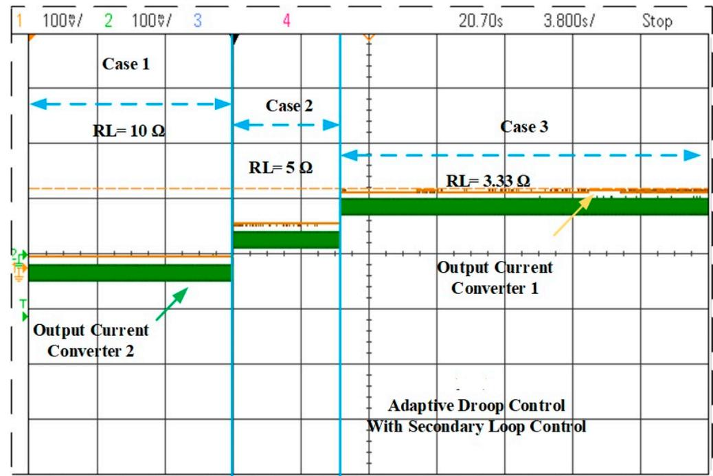
Figure 17. The output current of two converters at Adaptive droop gain with secondary control during load changes of 10 to 5 and 3.33 and input voltage changes.
