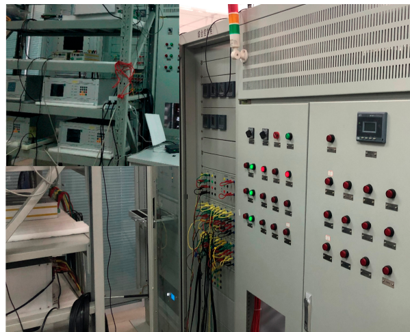
Figure 14. Dynamic simulation fault diagnosis experimental platform.
