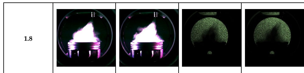
Figure 14. The images of the spray impingement by the piston.
