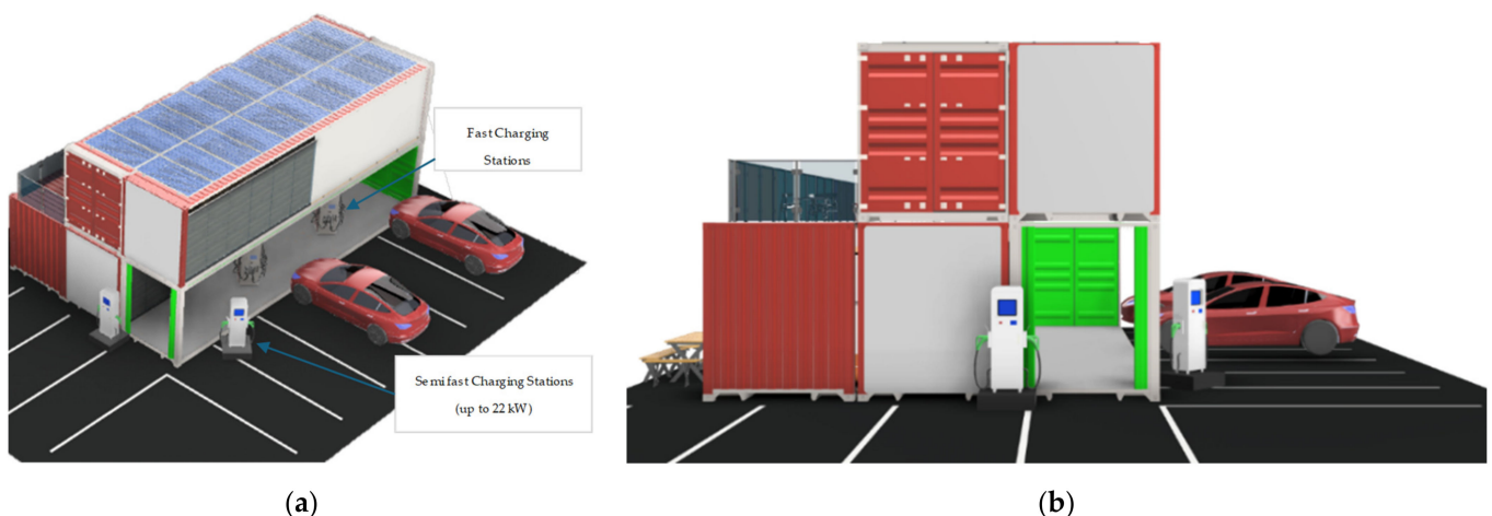
Figure 2. Conceptual model for an ideal EV charging hub: (a) With fast and semi-fast charging stations; (b) Model with allocation of semi-fast chargers (side view).
