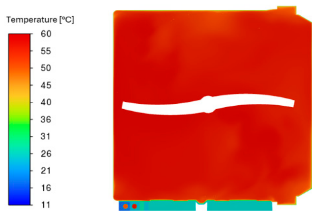
Figure 29. Temperature distribution in the XY section of the new heat exchanger and chamber.
