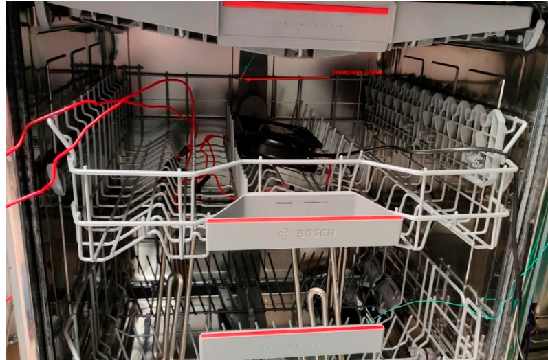
Figure 8. Experimental setup of the fan and heating elements inside the dishwasher.
