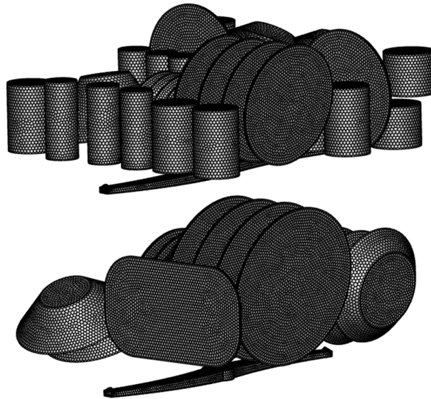
Figure 17. Finite volume mesh for chamber load and spray arm walls.
