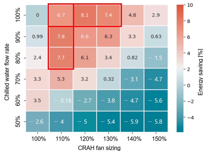
Figure 7. Energy sensitivity according to the changes in the CRAH fan air flow and chilled water flow.
