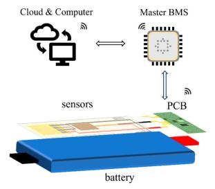
**Figure 1.** Schematic illustration of a smart battery equipped with multiple types of internal and external sensors.
