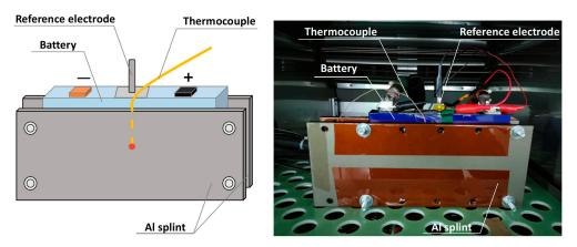
**Figure 2.** Sensing of internal electrode potential: high-capacity battery with built-in reference electrode and optimization of fast battery charging strategy based on reference electrode (reproduced with permission from Liu et al. International Journal of Energy Research; published by John Wiley and Sons, 2021) [16].
