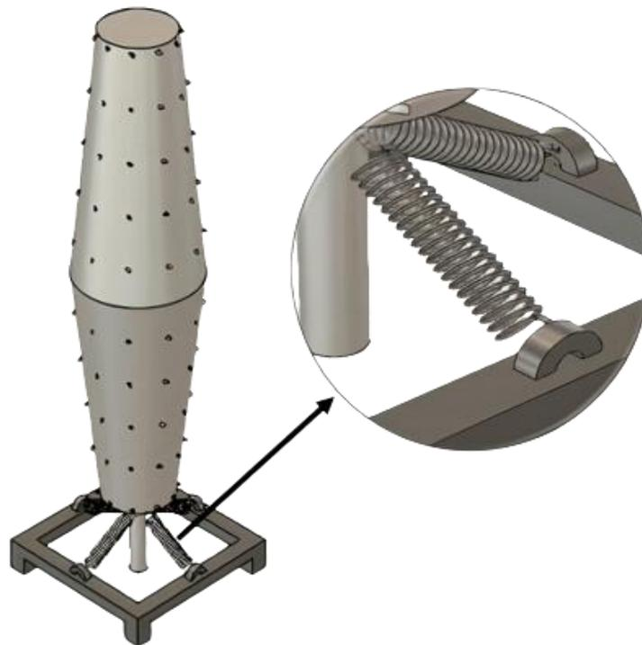
**Figure 5.** Schematic of a VBWT system with base and spring design. The above system is used for both models.
