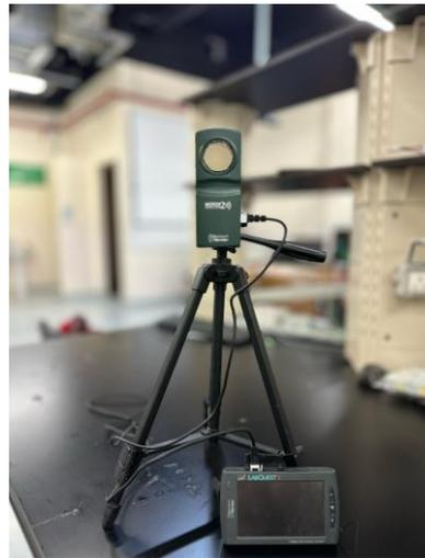
**Figure 14.** Ultrasonic motion-detection and measuring instruments are used to measure the displacement, velocity, and acceleration of the VBWT.
