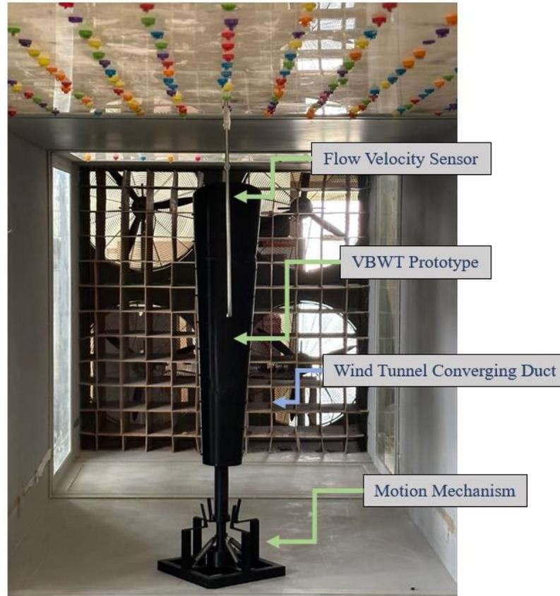
Figure 28. VBWT placement in the wind tunnel and the wind-flow-sensor attachment.
