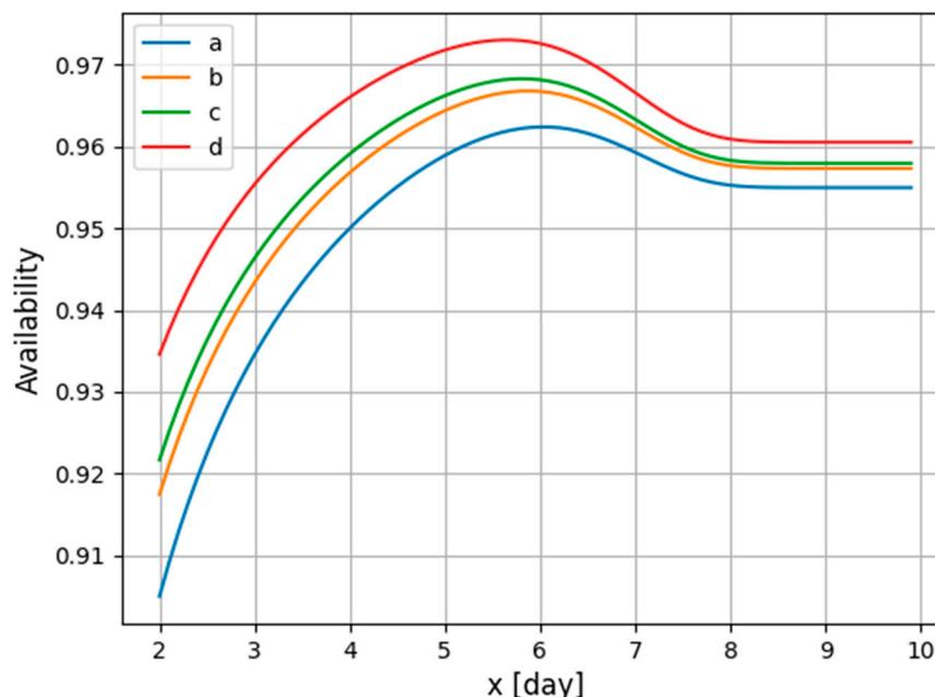
**Figure 6.** Function  $g(x)$  graph: availability of wind turbine in the function of time preceding preventive service  $x$  (day), marked when the frequency of preventive service is the same as in example 1 (line a) and in the case of shortening the period of preventive maintenance by 15%, 25%, and 35%, respectively, (lines b, c, and d).
