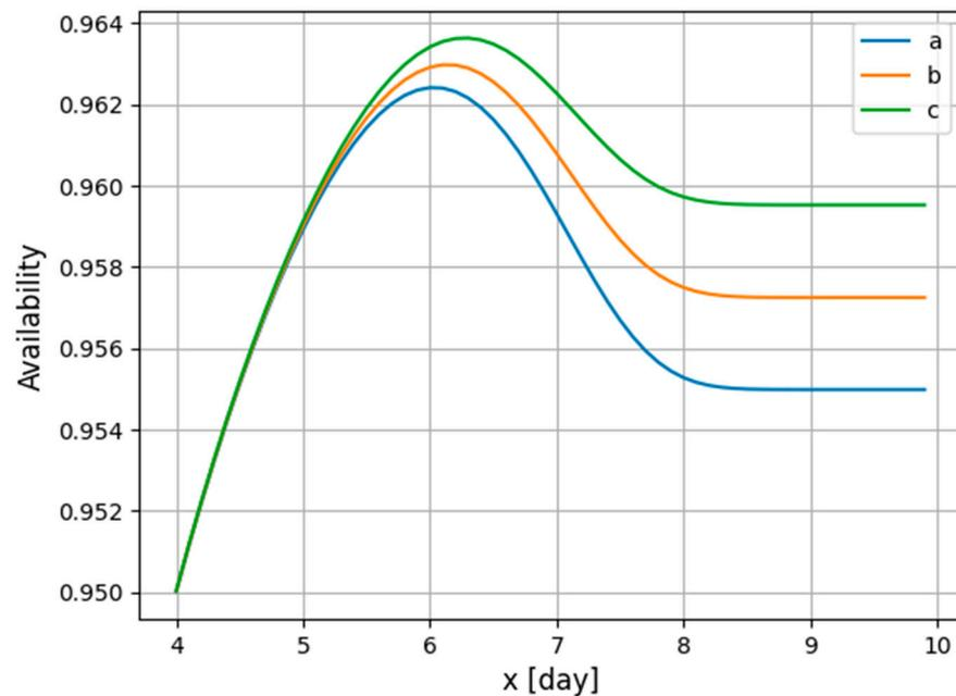
**Figure 8.** Function  $g(x)$  graph: availability of wind turbine in the function of time preceding preventive service  $x$  (day), marked for data from example 2 (scenario a) and scenarios b and c, for which the abilities of production and electric energy storing in state 2 of system modeling are estimated at 50% (line b) and 100% (line c).
