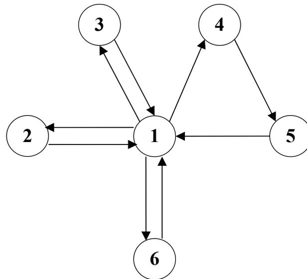
**Figure 2.** Illustration depicting state transitions in the preventive maintenance system model based on the age of Enercon E82-2 wind turbines, with the state  $S = \{1 \text{ to } 6\}$ .
