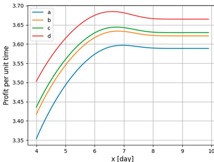
**Figure 5.** Function  $g(x)$  graph: profit over time (1k PLN/day) in the function of time preceding preventive service  $x$  (day), marked when the frequency of preventive service is the same as in example 1 (line a) and in the case of shortening the period of preventive maintenance by 15%, 25%, and 35%, respectively (lines b–d).
