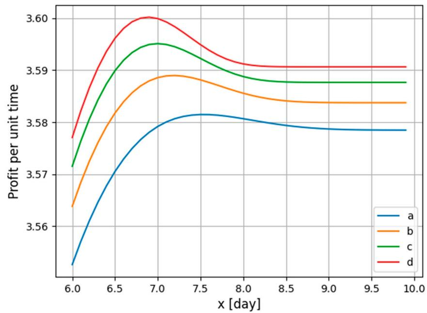
**Figure 3.** Function  $g(x)$  graph: profit over time (1k PLN/day) within the preventive service  $x$  function (day), marked for the Weibull distribution: shape = 6.5, 8, 9.5, 11, and scale = 8 (lines a–d, respectively).
