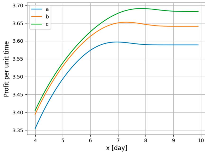
**Figure 7.** Function  $g(x)$  graph: profit over time (1k PLN/day) in the function of time preceding preventive service  $x$  (day), marked for data from example 2 (scenario a) and scenarios b and c, for which the abilities of production and electric energy storing in state 2 of system modeling are estimated at 50% (line b) and 100% (line c).
