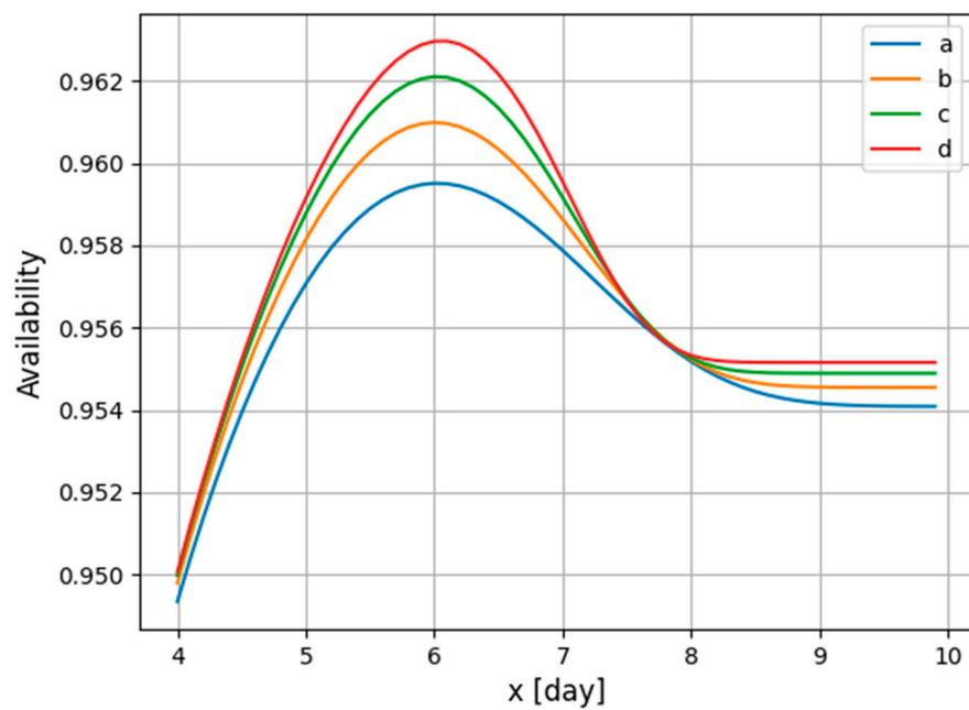
**Figure 4.** Function  $g(x)$  graph: wind turbine availability in the function of preventive service  $x$  (day) marked for the Weibull distribution: shape = 6.5, 8, 9.5, 11, and scale = 8 (lines a–d, respectively).
