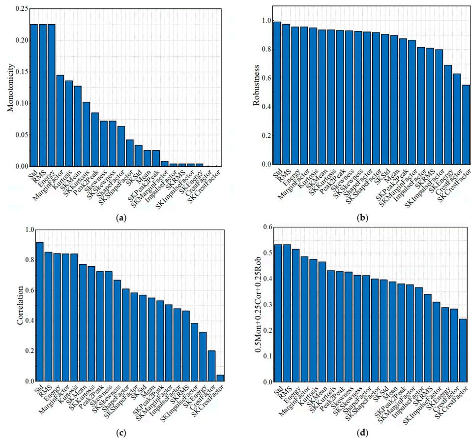
**Figure 2.** Indices performance metrics: (a) Monotonicity; (b) robustness; (c) correlation; (d) 0.5 Mon + 0.25 Cor + 0.25 Rob.
