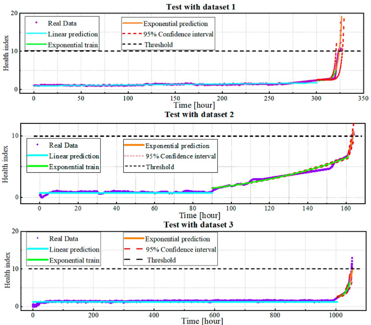
Figure 11. RUL prediction results of degradation models.
