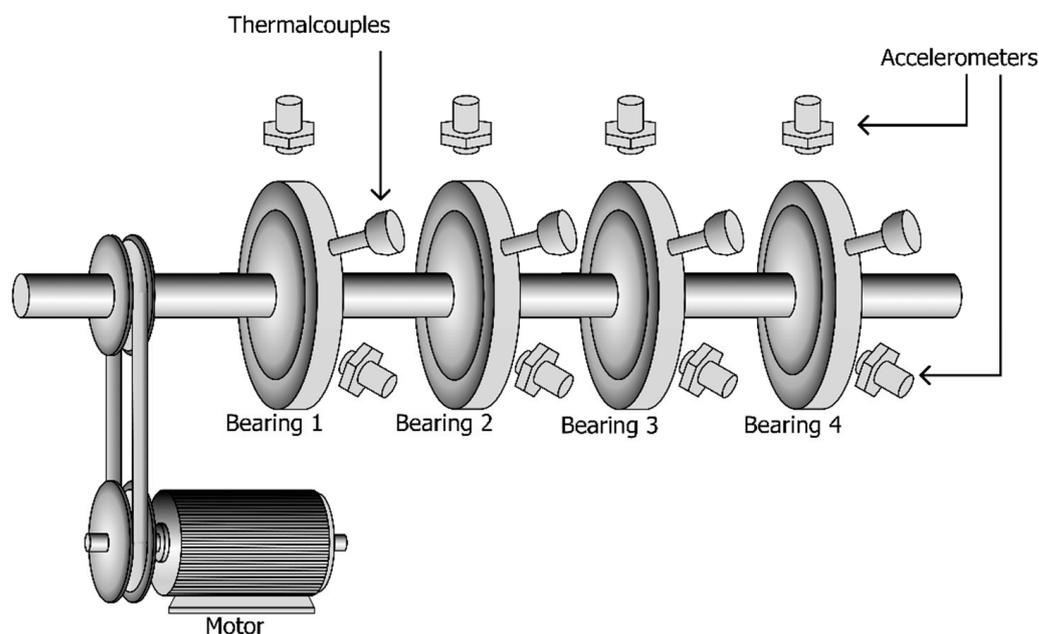
**Figure 1.** Bearing test rig.
