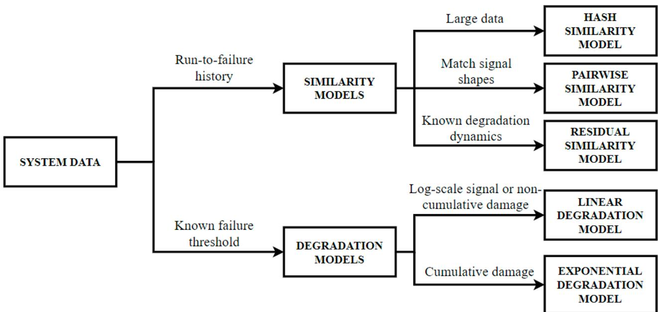
Figure 8. Approach to predicting RUL of main bearing.
