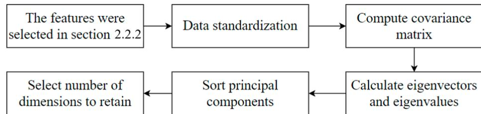
**Figure 3.** The process of determining HI from PCA.
