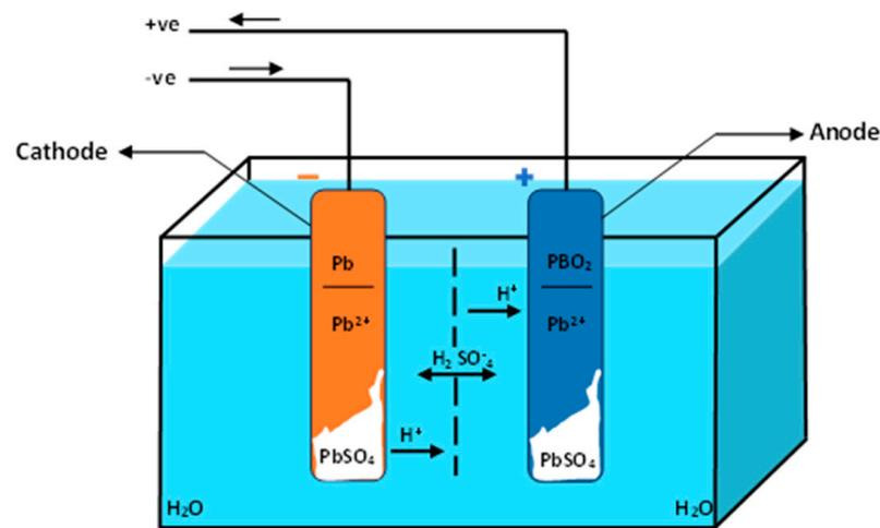
**Figure 2.** Schematic Diagram of A Lead-Acid Battery, adapted from [60].
