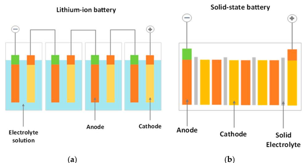
Figure 8. Lithium-ion battery (a) vs. solid-state battery (b) structures.
