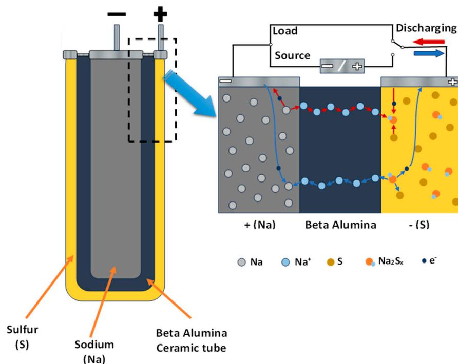
Figure 6. Sodium-sulfur NaS battery structure [73].
