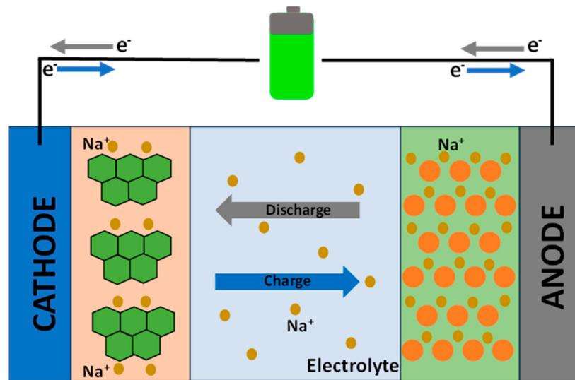
Figure 5. Schematic representation of a Na-ion battery cell [70].
