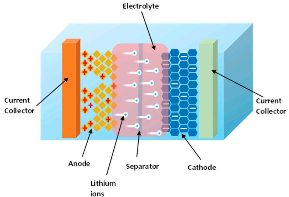
**Figure 3.** Lithium-ion battery components, adapted from [63].
