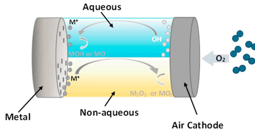
Figure 7. Metal-air battery structural form, adapted from [74].
