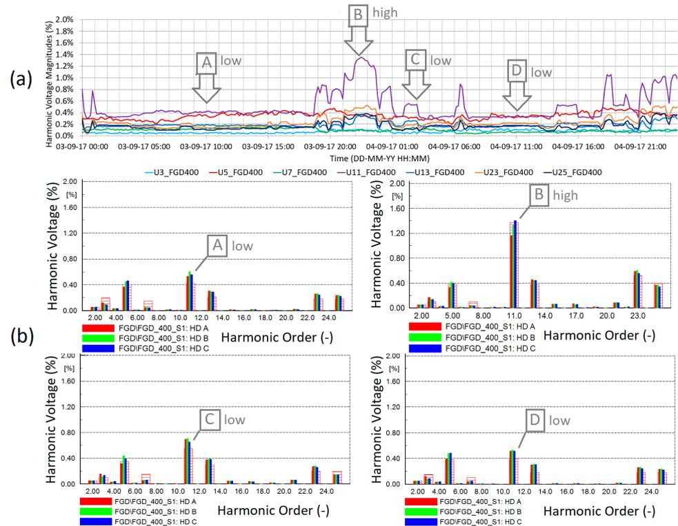
**Figure 9.** Comparison of (a) measured and (b) simulated harmonic voltages in the 400 kV substation Fraugde for the snapshots A, B, C, and D. The annotations ‘high’ and ‘low’ refer to the 11th harmonic voltage magnitudes.
