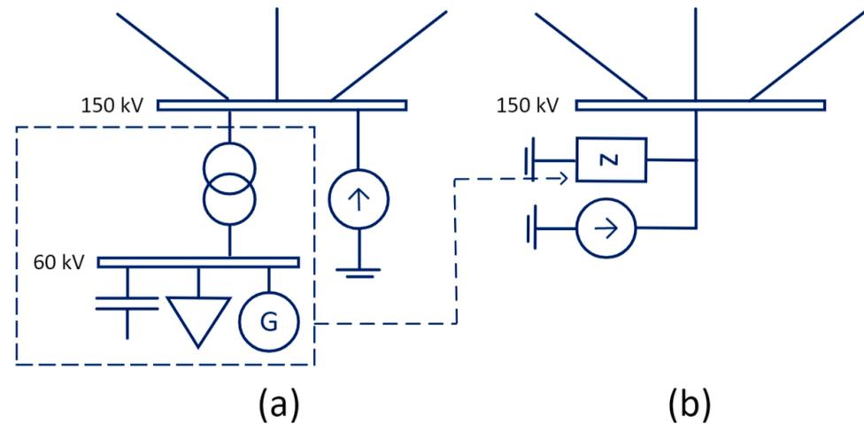
**Figure 3.** Representation of the network impedance of a distributed harmonic source: (a) passive harmonic characteristics of the 150/60 kV transformers, capacitance of the (cable dominated) 60 kV network, load and generation, (b) serving as the impedance in parallel with the harmonic current source.
