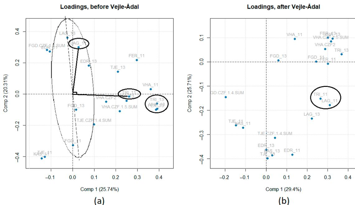
**Figure 19.** Loading plots for the data set containing aggregated values of 11th and 13th harmonic voltage and harmonic filter operation status. PC1 and PC2 are shown; (a) data before the Vejle-Ådal 400 kV UGC and (b) data after the Vejle-Ådal 400 kV UGC.
