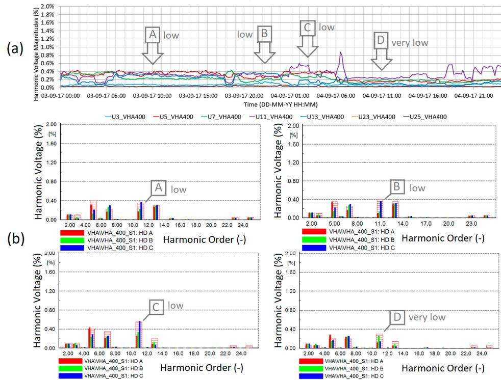
**Figure 10.** Comparison of (a) measured and (b) simulated harmonic voltages in the 400 kV substation V. Hassing for the snapshots A, B, C, and D. The annotations ‘low’ and ‘very low’ refer to the 11th harmonic voltage magnitudes.
