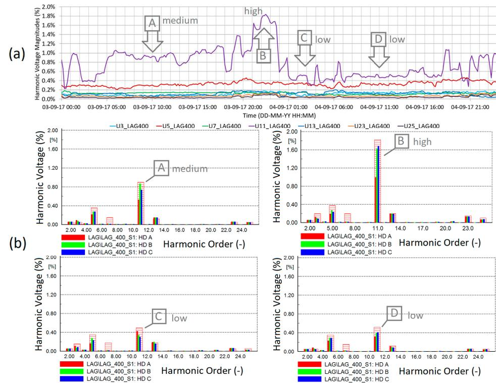
**Figure 11.** Comparison of (a) measured and (b) simulated harmonic voltages in the 400 kV substation Landerupgård for the snapshots A, B, C, and D. The annotations ‘high’, ‘medium’, and ‘low’ refer to the 11th harmonic voltage magnitudes.
