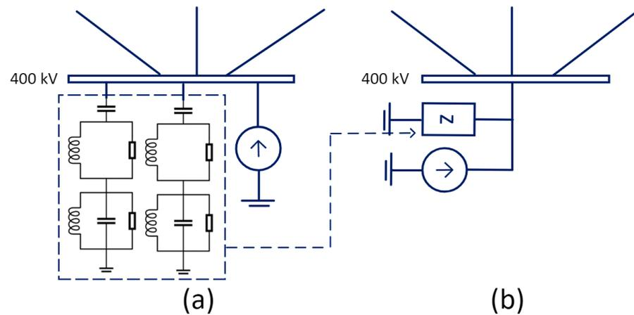
**Figure 4.** Harmonic representation of the HVDC Converter Station: (a) harmonic filter models in parallel with the harmonic emission source, (b) harmonic filters serving as the impedance in parallel with the harmonic current source.
