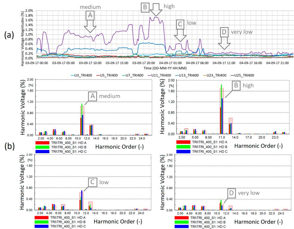
**Figure 8.** Comparison of (a) measured and (b) simulated harmonic voltages in the 400 kV substation Trige for the snapshots A, B, C, and D. The annotations ‘high’, ‘medium’, ‘low’, and ‘very low’ refer to the 11th harmonic voltage magnitudes.
