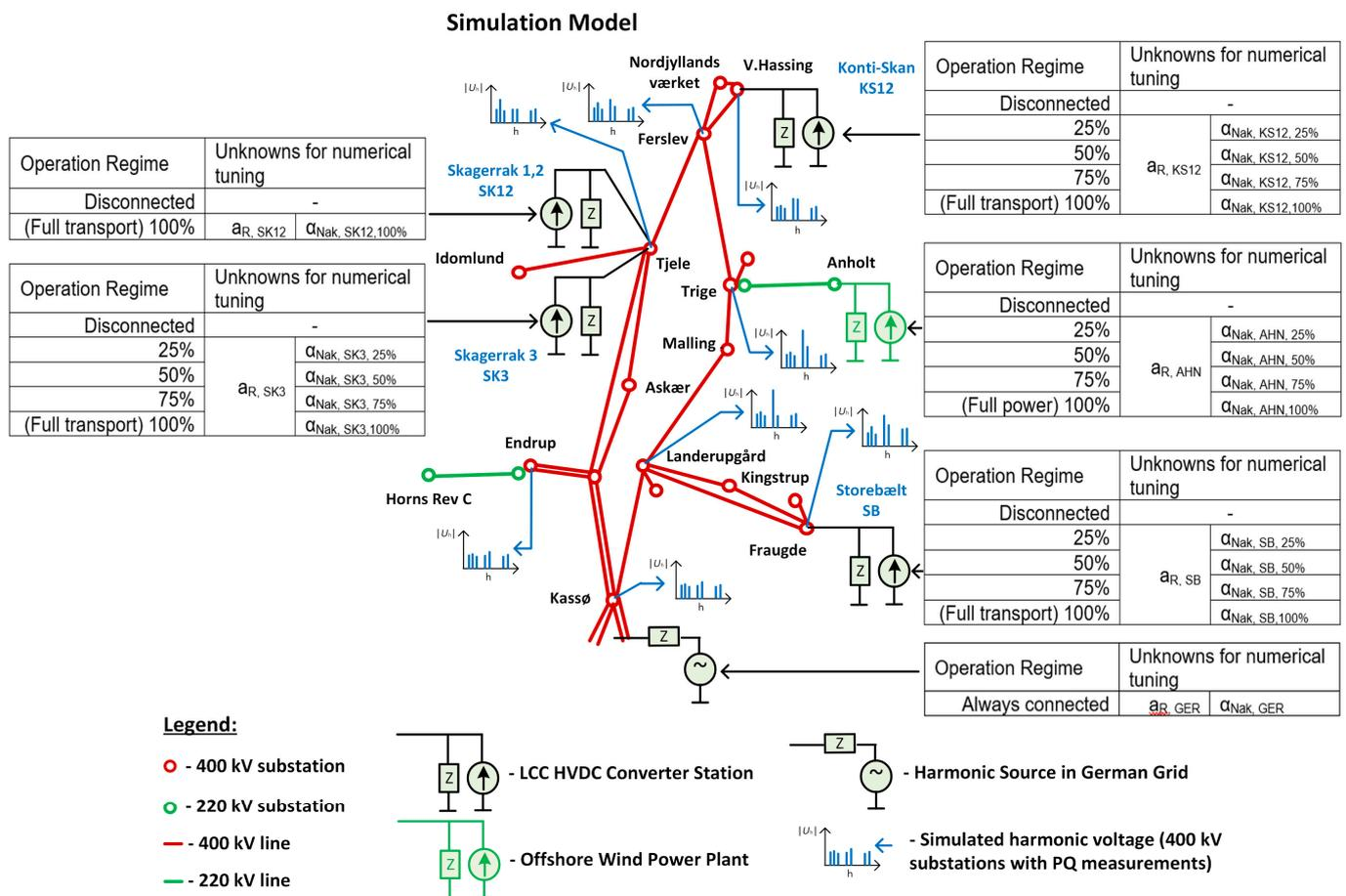
**Figure 5.** Application of the simulation model of the Western Danish 400 kV transmission grid for the numerical tuning of the relative components of the harmonic emission sources with notification of unknown parameters. The unknown parameters will be determined by the numerical tuning. The simulated magnitudes of the harmonic voltages are for the 400 kV substations with available harmonic voltage measurements at the time of the model development in 2020.
