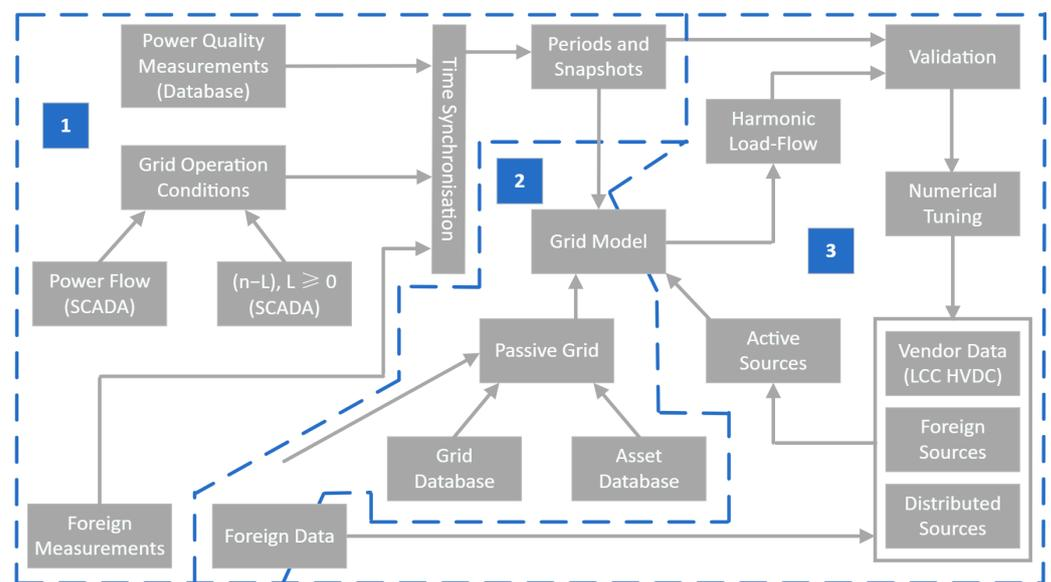
**Figure 6.** Development process of the model for direct simulation of harmonic voltage distortion in the 400 kV transmission grid of Western Denmark. The markings 1, 2, 3, show the process major steps.
