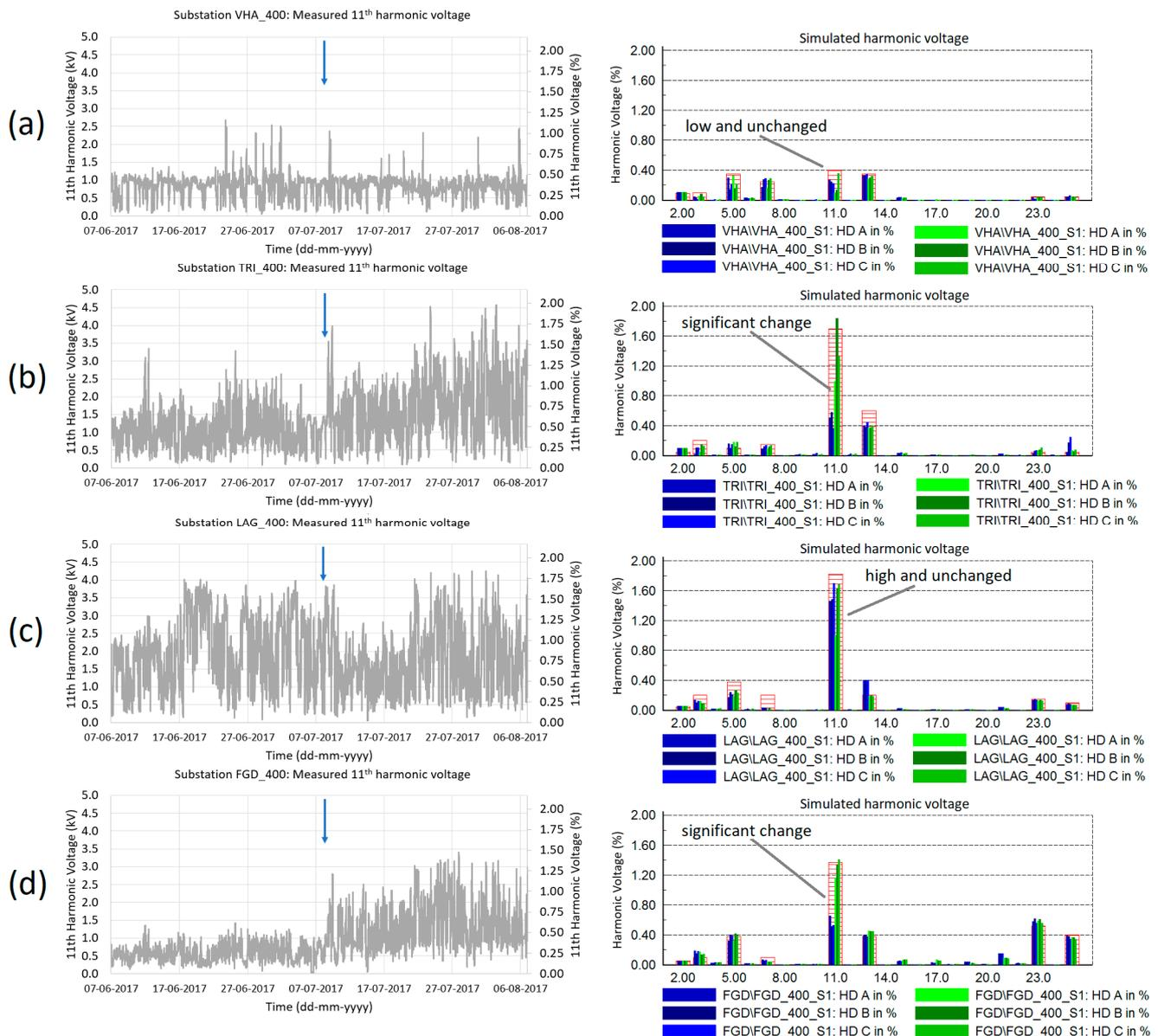
**Figure 16.** Demonstration of harmonic distortion prediction by simulation for the Vejle-Ådal 400 kV UGC project. The measured and simulated harmonic voltages about the time of energization of the Vejle-Ådal 400 kV UGC: (a) V. Hassing (small magnitude and not changed), (b) Trige (significant change), (c) Landerupgård (high magnitude and not changed), (d) Fraugde (significant change).
