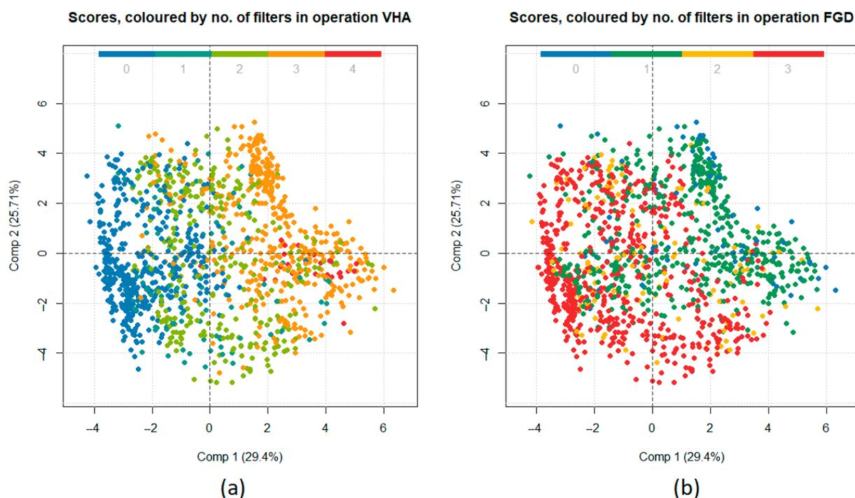
**Figure 20.** Scores plot for the data set containing aggregated values of 11th and 13th harmonic voltage and AC filter operation status. PC1 and PC2 are shown. Data after the Vejle-Ådal 400 kV UGC, (a) scores colored according to the number of AC filters in operation in V. Hassing, and (b) scores colored according to the number of AC filters in operation in Fraugde, are shown.
