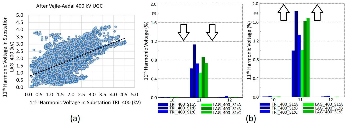
**Figure 17.** Positive correlation of the 11th harmonic distortion in the 400 kV substations Trige and Landerupgård in the present grid: (a) measurement with the linear tendency line by a dotted line, (b) simulations with blue histograms for Trige and green histograms for Landerupgård and the arrows showing the tendencies.
