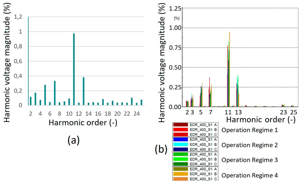
**Figure 15.** Comparison of (a) maximum 95th weekly percentiles of measured harmonic voltages and (b) simulated harmonic voltages in three phases in the 400 kV substation Endrup. The simulated operation regimes from 1 to 4 are present for giving the high magnitudes of the 11th harmonic voltage.
