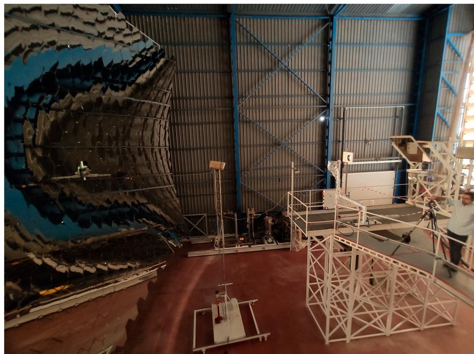
**Figure 2.** Photo showing the huge and multifaceted SF60 paraboloid concentrator (left) and a much smaller secondary reflector (with diameter of only 191 mm) positioned near the primary focal point.
